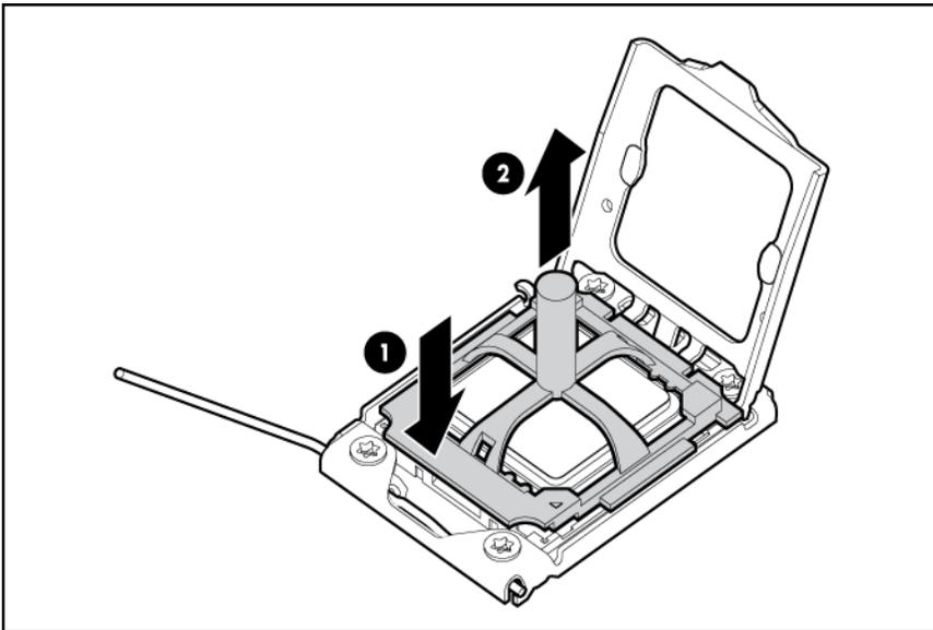
10. Close the processor socket retaining bracket and the processor retaining latch.
