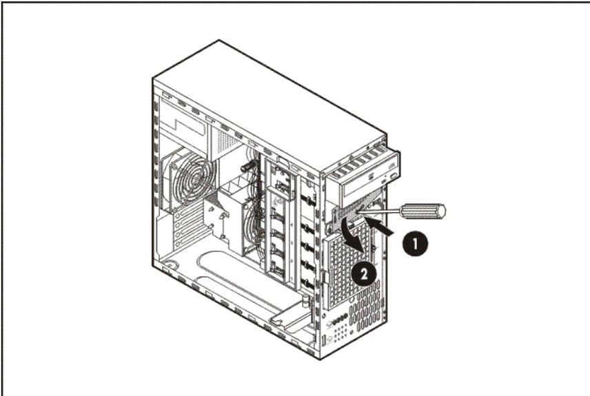
6. Install the four screws into the top screw holes on the media device.
