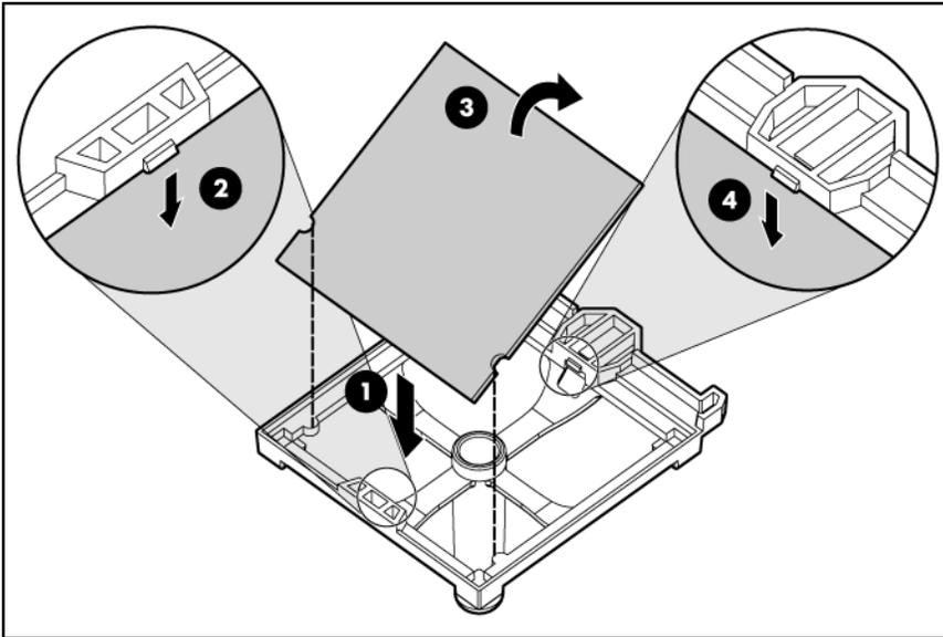
8. Align the processor installation tool with the socket and install the processor.
