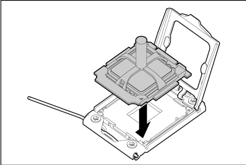
9. Press down firmly until the processor installation tool clicks and separates from the processor, and then remove the processor installation tool.
