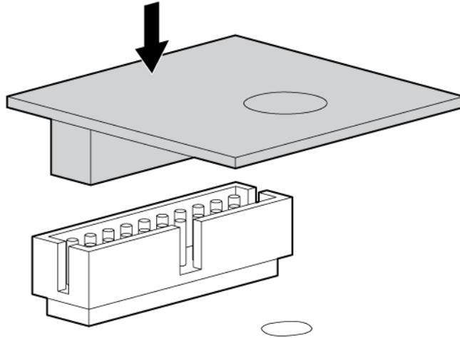
8. Install the TPM security rivet by pressing the rivet firmly into the system board.
