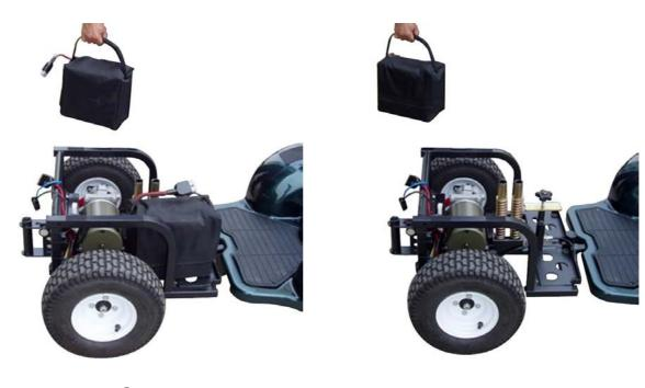
**Step 6**Remove Batteries
