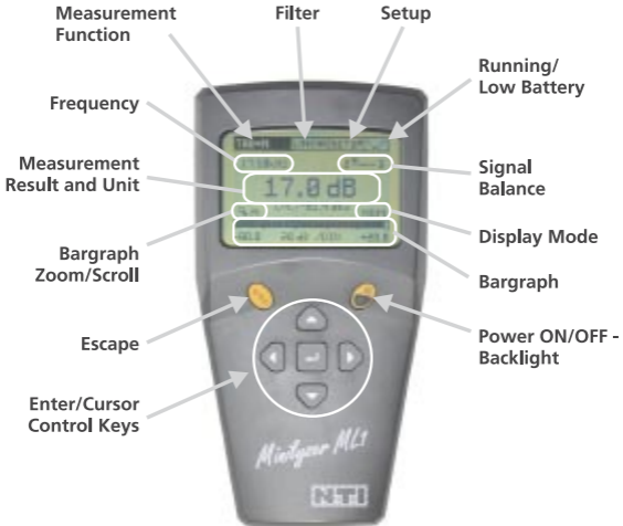
Fig 2.1 Display & Control Elements
