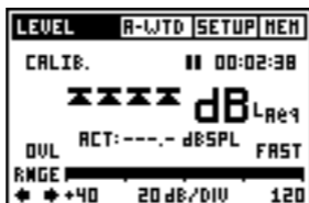
Fig 3.4 SPL Panel with Overload
