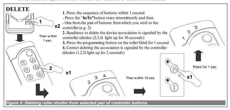
2. Removing a device ("EXCLUDE") from the Z-Wave network. A device excluded from the network does not have any number (Node ID) and can be included into another network. This state is signalled on the roller shutter by the network status diode (LED No. 2) which is illuminated permanently. The device is no longer a part of the network.
