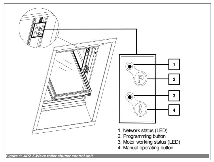
Figure 1 is presented an overall view of the available buttons and signaling, which is located in the upper right corner of the roller shutter.
