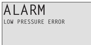
Regularly check the alarm indicator to ensure that the installation is working correctly. In event of alarm the heat pump will if possible supply heating to the house, primarily with the compressor, secondarily with the auxiliary heater. Hot water will stop to indicate that something noteworthy has occurred.
