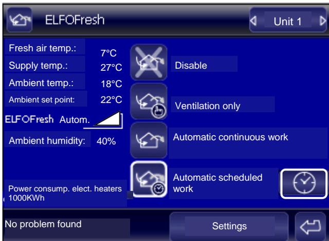
It sets the fresh air according to a daily hourly program, with a min. interval of 1 hour, in three operating modes:
