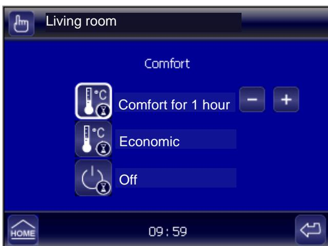
The min. setting interval of the predefined hourly program forcing is of 1 hour.
