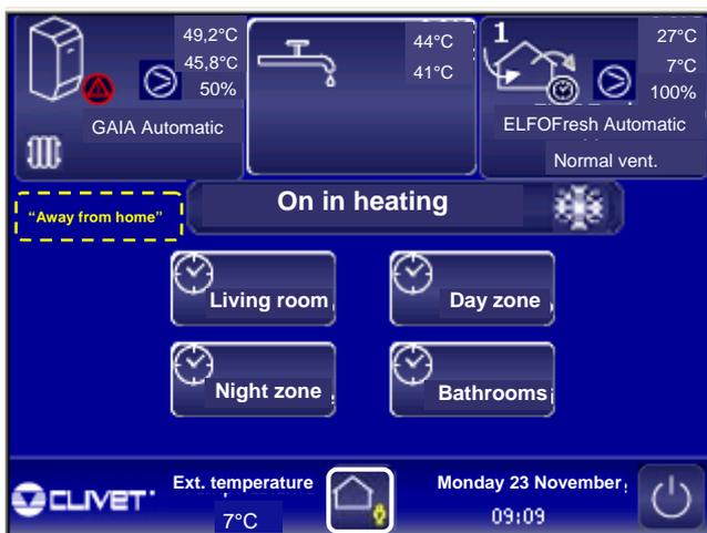
If is requested a different temperature in each zone of the house , this procedure must be repeated entering in each "Zone":
