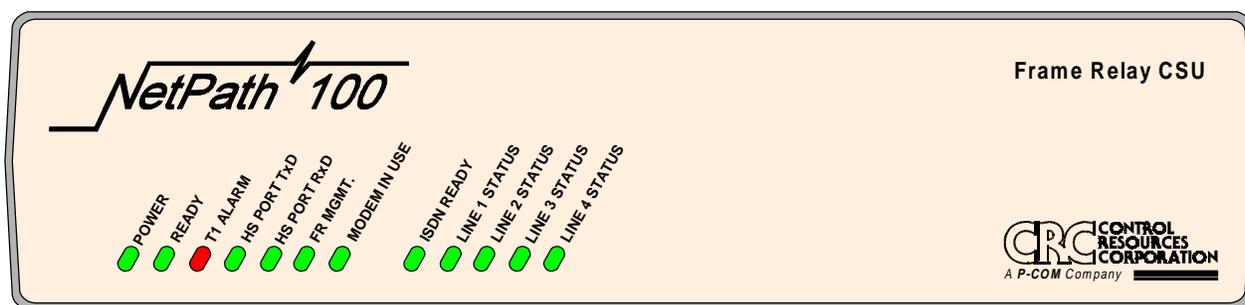
**Figure 6-7 NetPath 100 Front Panel with ISDN Adapter**
