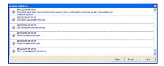
When connecting to the Unit, a comparison will be made between the configuration of the Unit which reflects the real system, and the configuration of the current project.
