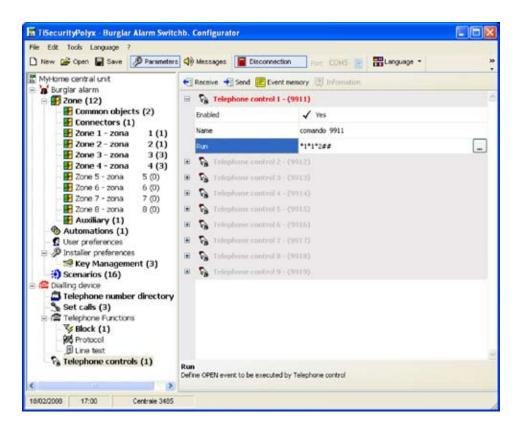
In this case, by remotely typing in the command 9911, the user will switch on the entrance lights whereas if 9901 is typed in, they will switch off.
