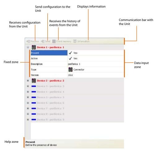
The upper bar includes the commands for communication with the control unit (only active when the connection with established PC); the central section is for data entry, and will vary depending of the selected parameter; the lower bar displays the instructions to guide the user through the data entry procedure.
