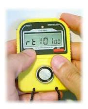
Hold the 'ESC' button and press the 'STOP/SELECT' button to select the Mode, Software version or the Serial number.
