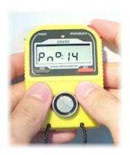
Enter the configuration menu, select 'P n°' function and press the 'ENT' button.
