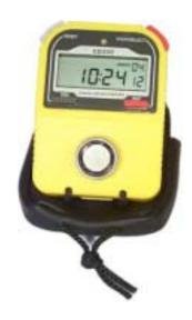
The Rally Timer is a microcomputer mounted inside a stopwatch body which is fitted with an ibutton interface.
