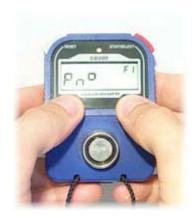
To enter the configuration menu, press both the 'ESC' and 'ENT' button.
