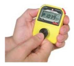
When the control worker presents, the ibutton to the Rally Timer, the first time into the queue is recorded into the ibutton and erased in the Rally Timer's embedded memory.
