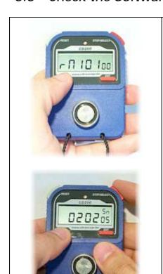
Hold the 'ESC' button and press the 'STOP/SELECT' button to select the Software version or the Serial number.
