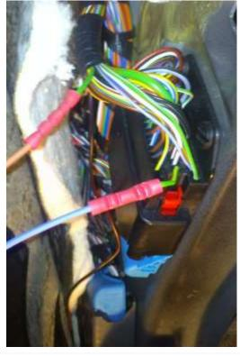
Connect both sides of the cut wire with shrink tubes with the following cables from the dLightBox:
