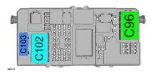
Connect the following 4 cables from the dLightBox through Scotchlok connectors with cables from connectors C96, C102 or C103 as described below (By disconnecting connectors C96 and C102, you can easily see the pin numbers at the bottom):
