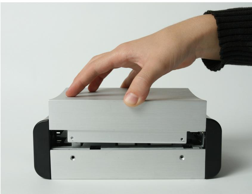
Figure 1.3: Opening the KNR-100 housing
