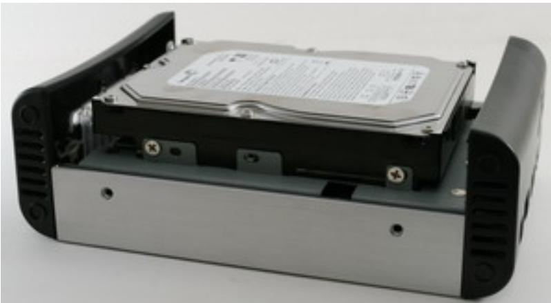
Figure 1.5: Correct securing of the hard disk in the KNR-100
