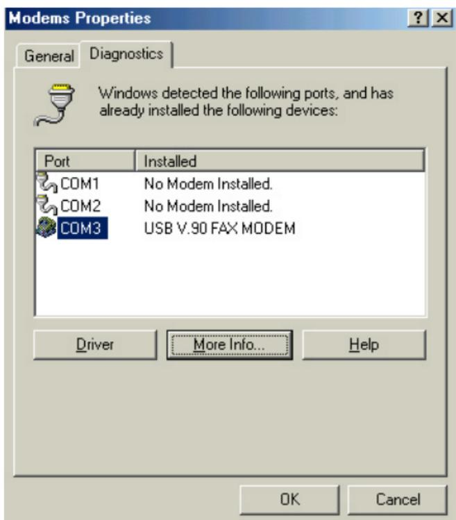
5. If the following information can be found, it means that the USB modem is well installed and enabled. Click **OK** to exit.
