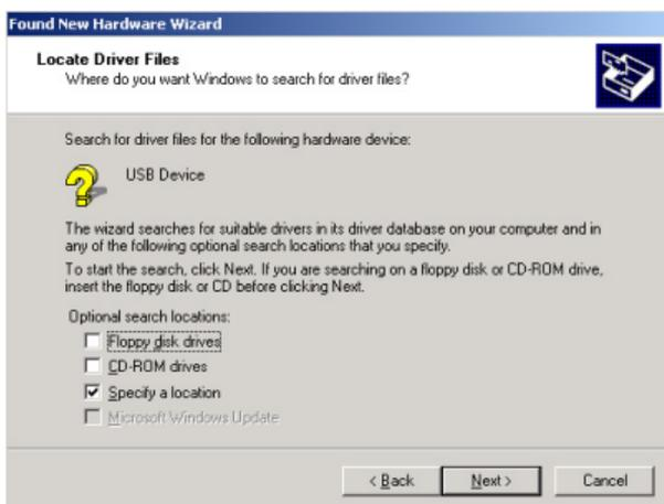
4. Type: **E:\WIN2K** (E is for example the drive where your CD-ROM is installed). Click **OK**. Windows will start searching for the appropriate driver for the software installation.
