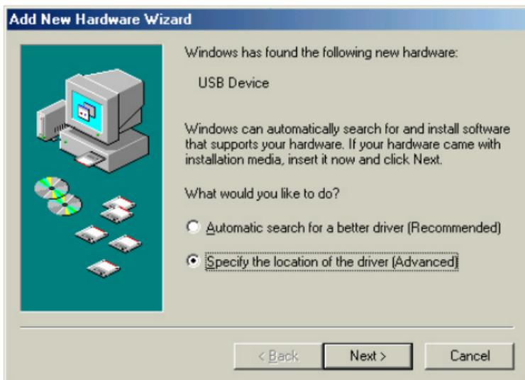
2. Load the device driver compact disc into the CD-ROM of your system and select **Specify**
