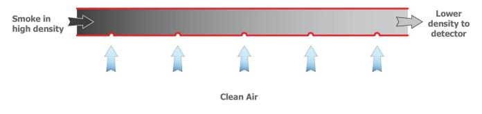
With micro-bore systems there are no side sampling holes to let in clean air. The dilution occurs at the detector when the pipes come together. If an FT15 is being used with all of its fifteen pipes sampling then each pipe brings in 1/15th of the sampled air (assuming a balanced system). The number of pipes is directly related to the fraction of the total air that is sampled making calculations more straightforward than with wide-bore systems.
