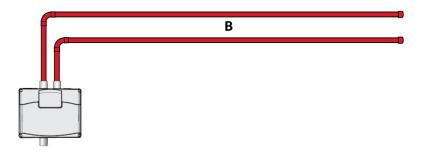
Type 2 layout, T-pipe, both pipe runs each side of the T junction can go up to 100 m (A+B). For detailed planning, check application with PipeTracer.
