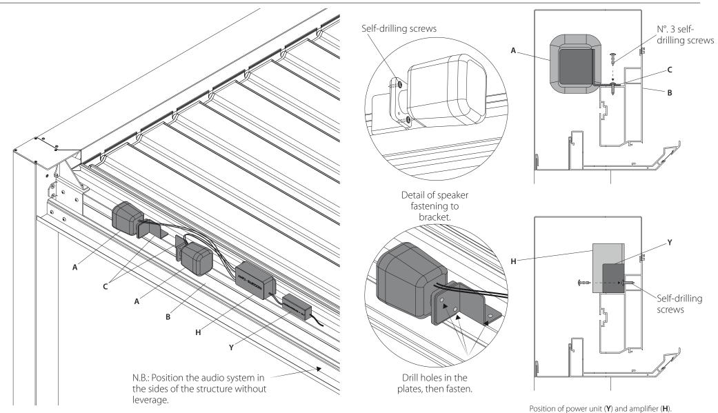
**fig. 1**Fasten the two speakers (**A**) to supporting profile (**B**) using brackets (**C**), positioning them as shown in the figure.
