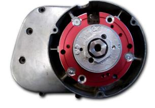
It is possible to embed the ignition into the housing, so the ignition doesn't stick out as much. This may be done to avoid the ignition scraping the ground while going through corners.
