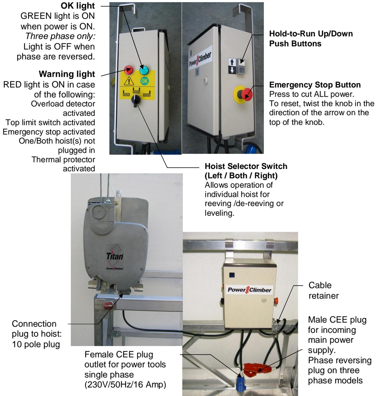
The TITAN hoist is a self-reeving traction hoist, powered by an electric motor. The hoists and the central control box (CCB) are mounted on Temporary Suspended Platforms (TSP) and suspended with steel wire ropes from a suspension system. The strength of the platform and the suspension system used in combination with the hoists must be in relation to the Working Load Limit (WLL) of the hoist.
