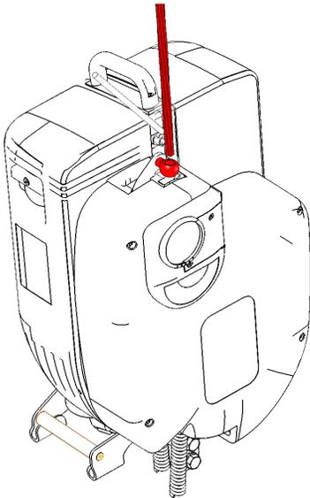
1. Push back the slack rope lever and insert the suspension rope through the eye of the slack rope lever and into the hoist until it stops.
