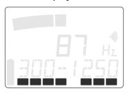
The volume display indicates the volume set. If the bar on the extreme left is shown in reverse video, the volume is low; if the bar on the extreme right is shown in reverse video, the volume is maximum.
