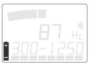
The battery symbol appears about 15 minutes before the battery runs out. In case the accumulator volume drops further, the instrument automatically switches off to protect the accumulator.
