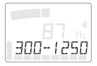
Different leak noises can be heard best in different frequency ranges, and two people may hear the same noise differently. To optimise acoustic perception a bandpass can be set. In this case only a particular frequency range is fed to the headphones. The best setting can be found by experiment, or alternatively the **A 100** can search for it automatically.
