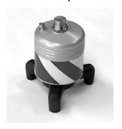
The ground microphone 3P-4 is used to locate leaks beneath unstabilised surfaces. An earth spike can be screwed onto it for use in soft ground. Its 3 feet guarantee stability at all times.
