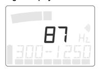
The digital display indicates the smallest value measured during a single measurement.
