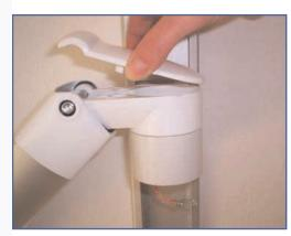
8. Remove the right hex screw M 6 x 12 and replace it with the hex key M 6 x 40. Fasten the screw until the depth gauge without using any force.
