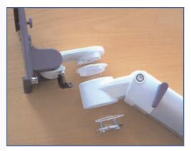
4. Remove the outer cover form the outer pivot block by loosing the (2) socket head screws M 5 x 20.
