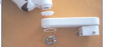
5. Put the spiral cable wrap into the support arm profile and turn the console back by 180° to its original position.
