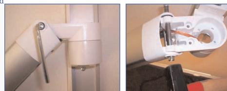
WARNING: Avoid pulling out the spindle completely.
