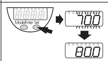
Numerical values are incremented continuously. For reducing the value: Let the display move to the maximum setting value. Then the cycle starts again at the minimum setting value.
