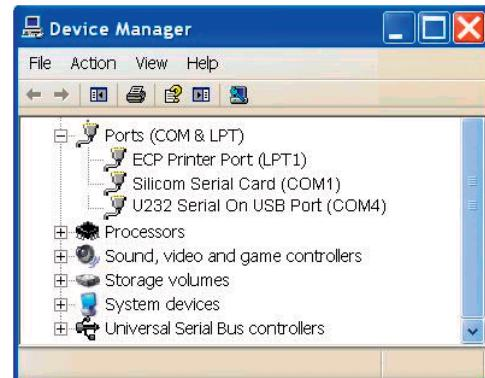
This example shows the COM ports of a PCMCIA card and a USB-RS232 converter:
