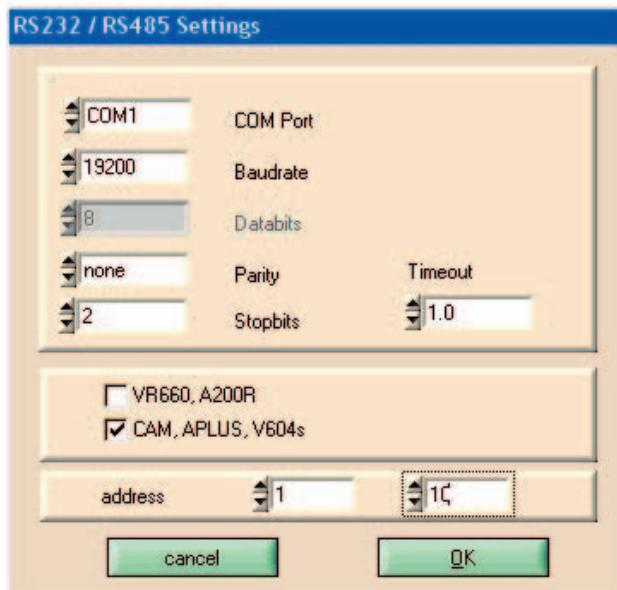
The existing COM ports are determined as the communication interface when starting the program and selecting RS232/RS485. Only COM ports found are available for selection.
