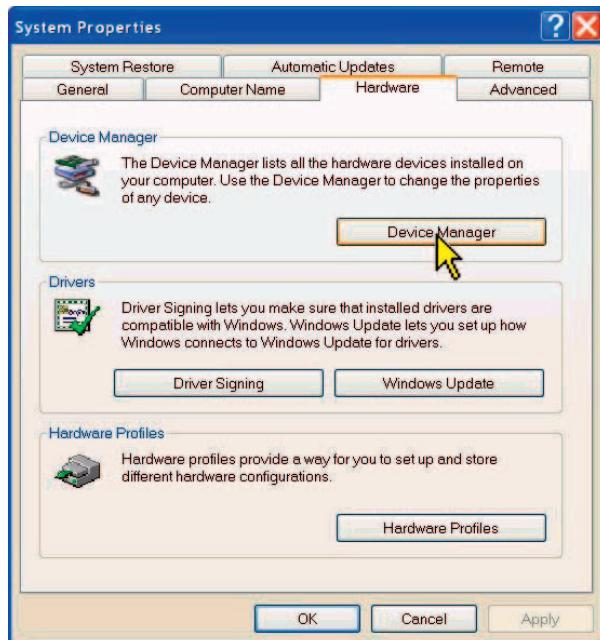
The COM port of an external RS232 or RS485 converter may be determined (and, if required, changed) via the Windows system control.
