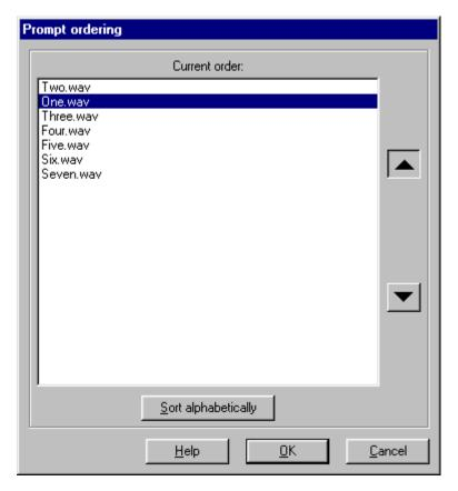
Pressing the up- and down-arrow buttons moves the selected file up or down in the list. You can keep those buttons pressed to move a file over a long distance in the list.
