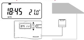
The Remote Temperature Sensor accessory can be fitted to your Chronotherm to control the temperature of another room where it is inconvenient to locate the Chronotherm e.g. commercial premises where the public may adjust buttons.
