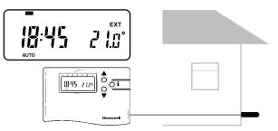
The Outside Temperature Sensor accessory can be fitted to your Chronotherm to display the outside temperature. By pressing the INFO 1 button twice, the Chronotherm displays the external temperature.
