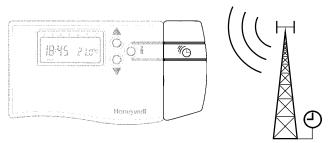
The ATS module picks up a daily time signal from a transmitter in Central Europe and corrects the time on the Chronotherm display. So:
