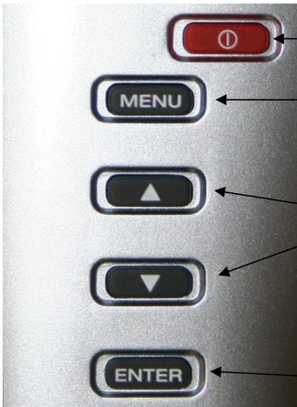
**ON/OFF:** Turns the instrument on or off. (Press briefly on this key)
