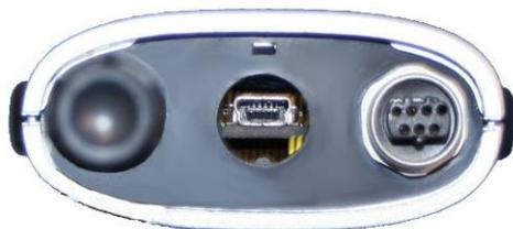
The service connector is a USB port and can be accessed without opening the enclosure after removing the protective red round cover.
