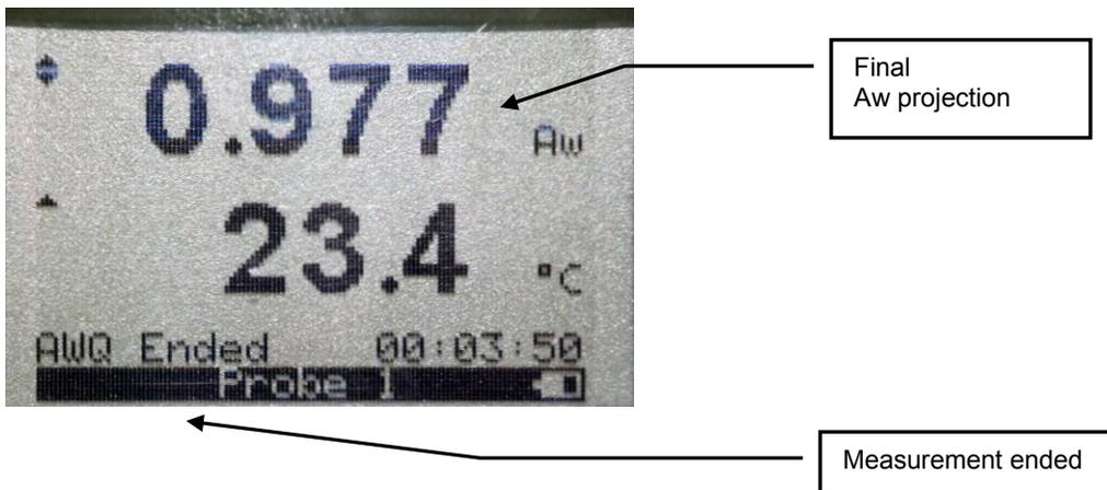
**5. AWQ Reset:** write down the measurement for each probe and press ENTER. The HP23 is ready to start a new measurement
