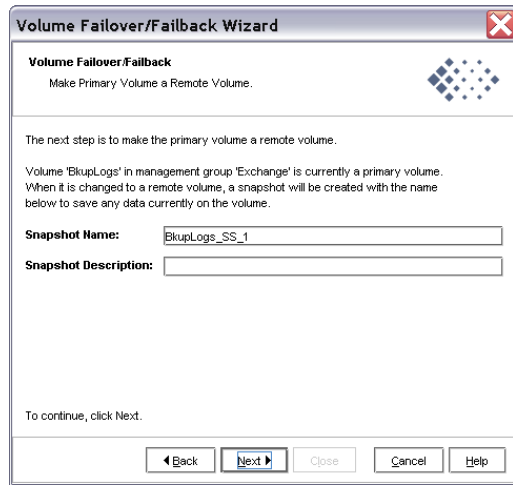
Figure 2.20. Creating a snapshot before making a primary volume into a remote volume
