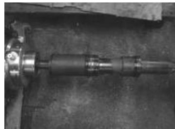
The greased ball screw assembly should appear very similar to the one shown above.
