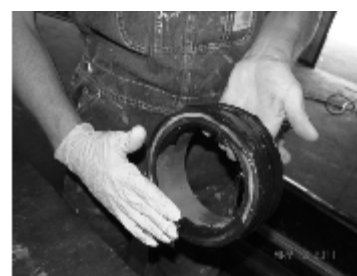
Then, grease and insert the external seal rings into the seal ring groove of each of the seats.
