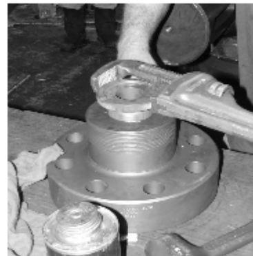
Tighten the packing retainer with a pipe wrench as shown.
