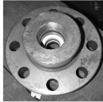
Insert a packing set into the bonnet as shown, and push it down.
