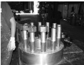
A stud-tightening nut will be used to tighten the studs.
