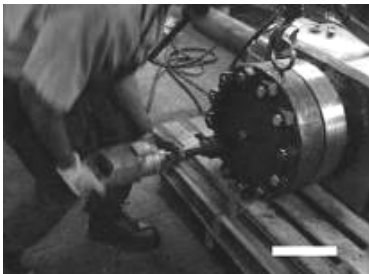
Torque the service flange hex nuts with a certified torque gun until they are tight.
