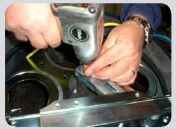
Turn the head over again and loosen the central bolt holding the filter shaker shaft.
