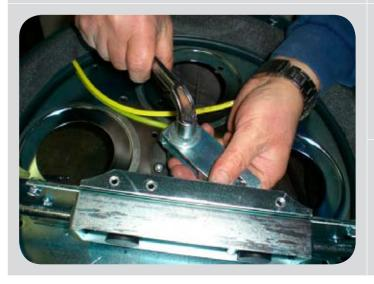
Hold the shaft while you unscrew the bolt.
