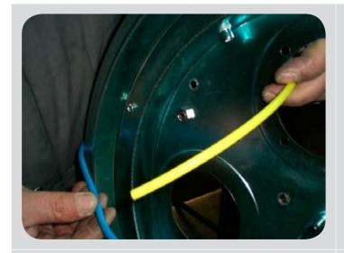
Make sure the pipes are in the right position. Yellow on the inner D.6x1/8" fitting, blue on the external D.6x M5 fitting.
