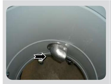
The deflector must be turned to the correct position (towards the container below).
