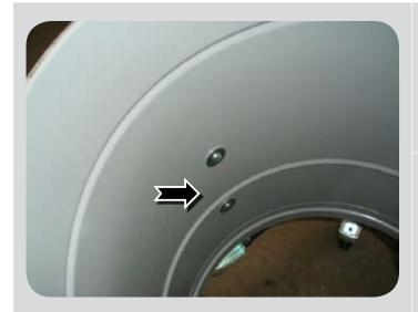
The roundhead screws must have a washer and be tightened down correctly to prevent air leaks (vacuum loss).
