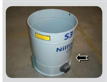
The complete inlet must be installed correctly (with the seal between the inlet and the filtering chamber and the screws tightened properly).
