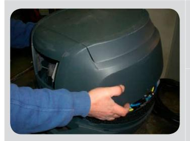
Hold the bottom edge to remove the motor cover. Pull the cover out, then up.
