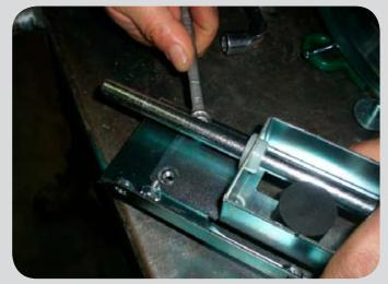
To dismantle the filter shaker system, unscrew the 4 screws holding it on the plate.
