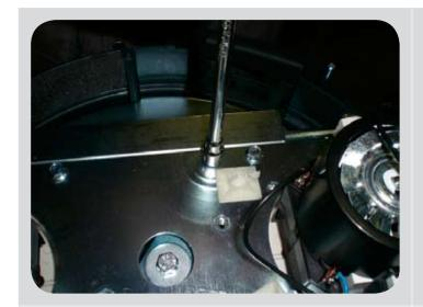
Proceed by removing the motor mounting plate. Unscrew all the hex-head M6 screws on the motor mounting plate using a hex-head wrench .
