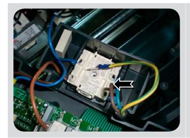
Always make sure the Faston terminals have been crimped correctly.
