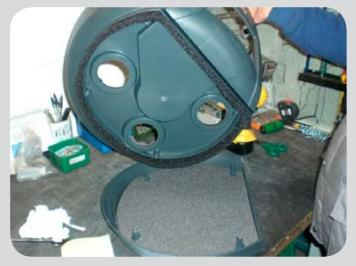
Remove the motor cover from the top cover.
