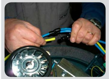
Pull the press-fit pipes off the connectors.
