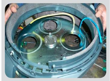
Remove the base of the motor cover from the motor mount.
