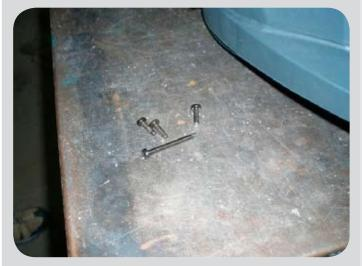
All the screws are the same length, except the one under the main switch which is much longer.
