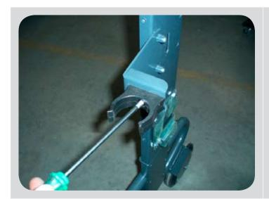
To remove and replace the plastic retainer of the accessories support, unscrew the screw in the centre.
