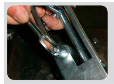
To remove the 2 bumpers, unscrew the 2 bolts holding them on the frame with a hex-head wrench.
