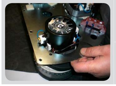
Pull the motor through the hole in the plate.
