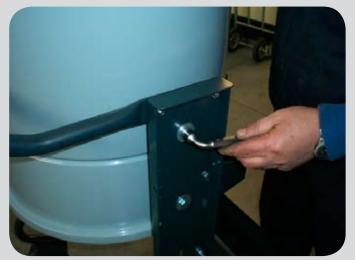
Use a hex-head wrench to loosen the top screw holding the side bracket.
