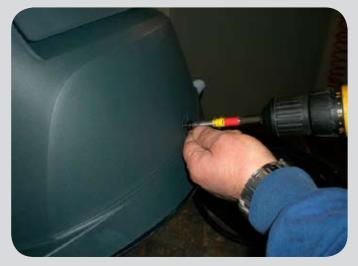
Unscrew the 4 screws positioned every 90° around the motor head.
