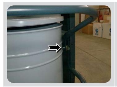
When inserting in the container, check the roller pin is inserted properly and slides freely on the coupling guide mounted on the uprights.
