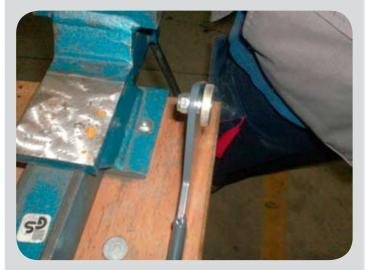
Remove the whole lever, opening it out so it comes off the 2 welded pins.
