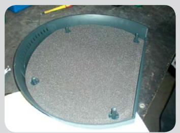
If you have to bond parts of the sponge that have come unstuck, clean the surfaces thoroughly and only then stick the sound-proofing sponge back on using a few drops of liquid glue.
