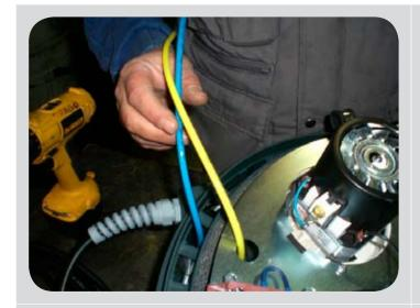
Pass the cables and tubes through the right holes.
