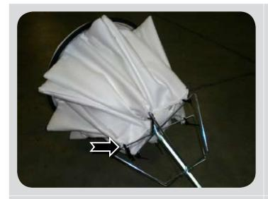
When the complete filter kit has been removed from the motor head, unscrew the clamp and remove the filter ring. Turn the filter upside down. Cut the plastic ties and detach the cage from the filter.
