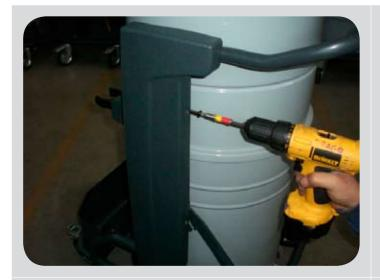
Unscrew the 4 screws fixing the upright side panel by hand or with a screwer.
