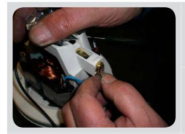
Pull downwards and disconnect the Faston terminal with the blue wire on the brushes.
