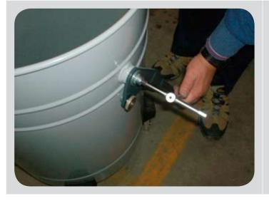
To remove the release lever, use an Allen wrench to unscrew the hex-head screws in the bush welded on the container.
