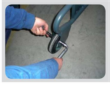
To remove and replace the fixed wheels, unscrew the nylock nuts with a wench.
