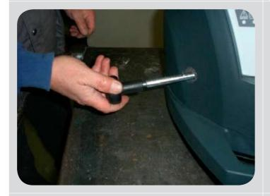
Proceed by unscrewing the filter shaker knob.
