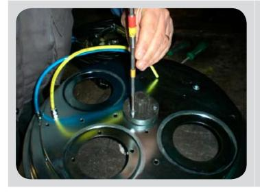
Unscrew the 3 screws holding the central bush on the motor mount.
