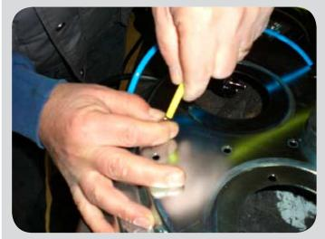
The pipes are press-fit in the fittings.
