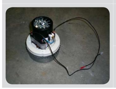
The power wires are already connected to the single-phase motor.
