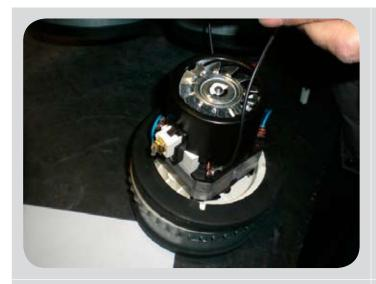
Once removed, the motor has 2 seals (top and bottom) on the fan.
