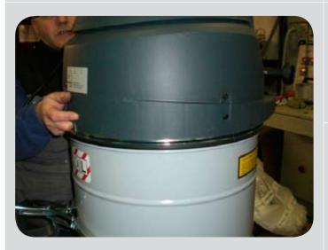
Remove the whole motor head, lifting it our of the frame, making sure you have a firm grip on it. Use the handles on the sides of the motor head.
