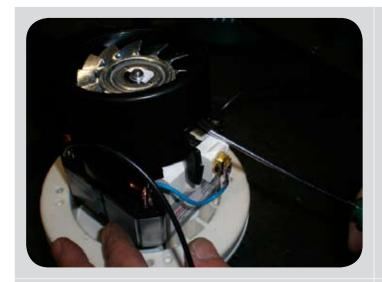
To change the brushes, bend and release the tab holding the motor cap.
