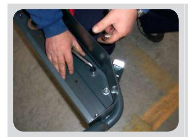
To remove and replace the accessories rack, unscrew the bolts under the front of the trolley.
