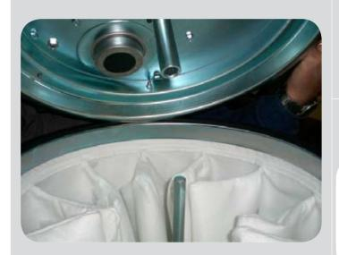
Remove the motor head, pulling out the hex-pin cage from the bush.
