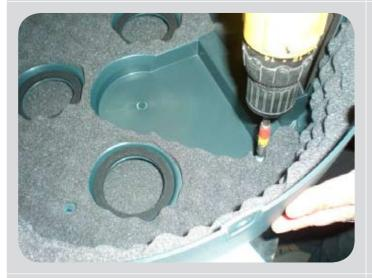
Turn the motor cover over and unscrew the screws inside.
