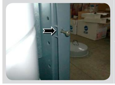
The longer screws must be used near the reinforcing spacer in the side-panel.
