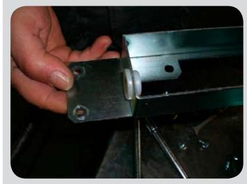
The 2 bushes must be press-fit and inserted from the outside in the holes on the box.
