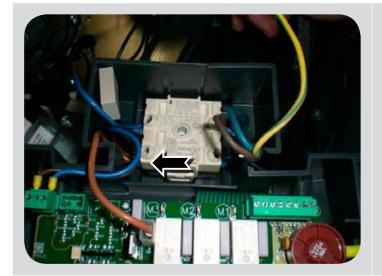
Remove also the cables going to the terminal board and those connecting the switch to the components of the electronic board.
