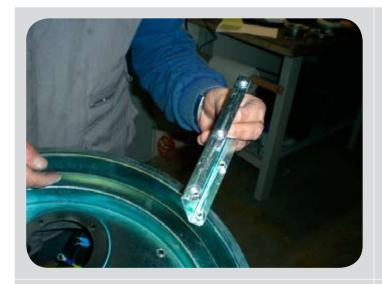
Turn the motor head over and remove the 2 spacers.
