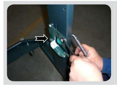
To remove and replace the container coupling bracket, unscrew the bolts with a hex-head wrench.
