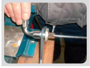
To remove and replace the roller pin, use a screwdriver and a hex-head wrench.
