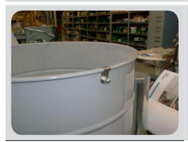
Make sure the tongue that guarantees earth continuity between the motor head the filtering chamber is always fitted.
