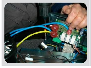
Unscrew the screws at the sides of the board.
