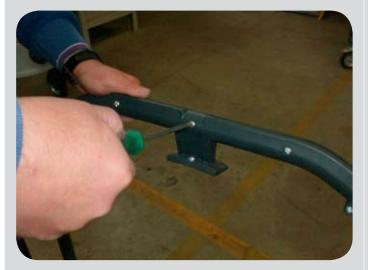
To remove and change the cable carrier, unscrew the 6 screws holding it on the handle.
