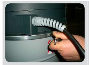
Open the closing band to remove the motor head from the filtering chamber.
