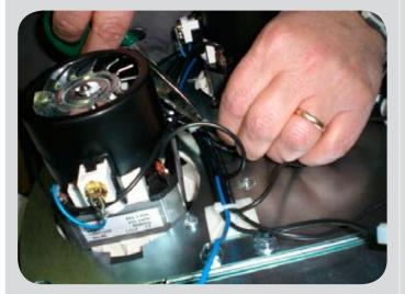
Remove the ties holding the cables on the motor mounting plate to make wiring easier.
