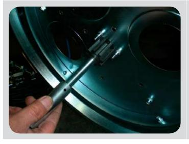
Turn the motor mount and pull the filer shaker shaft out of the central bush.
