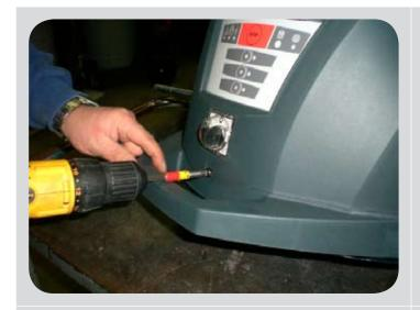
Remove also the screw under the main switch.
