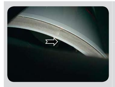
The seal must be fitted correctly in the side groove and bonded in place with suitable glue (such as Bostik). Also make sure the joint of the 2 parts is bonded properly.
