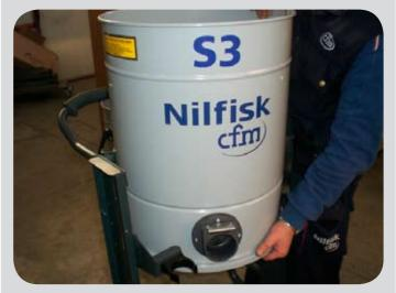
Remove the 4 screws holding the 2 side brackets, turn the filter chamber and pull it out of the 2 trolley uprights.
