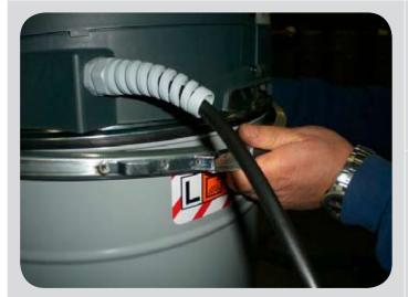
Open it out completely to remove it from the side link.
