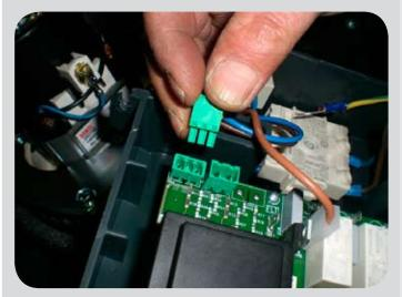
Pull off the green connector and connect the blue and brown wires to the board.
