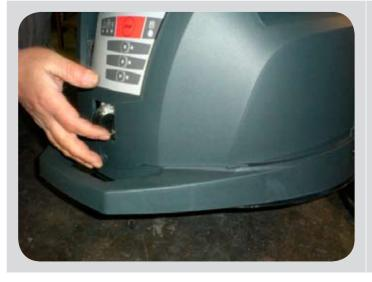
Now the motor cover can be removed from the base. Take particular care with the main switch. Pull it out, removing also the control panel.
