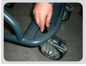
Remove the protective plug to remove the castors.
