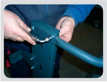
Proceed by unscrewing the handle with the cable carrier. Use a hex-head wrench to tighten the 2 screws on each side of the handle.
