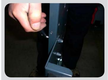
To remove and change the accessories support, unscrew the 2 screws holding it on the upright with a hex-head wrench.
