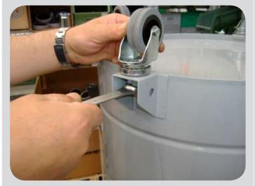
Unscrew the bolt in the wheel bracket using a hex-head wrench.
