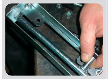
To remove the filter shaker shaft, pull it out from one side of the bush.
