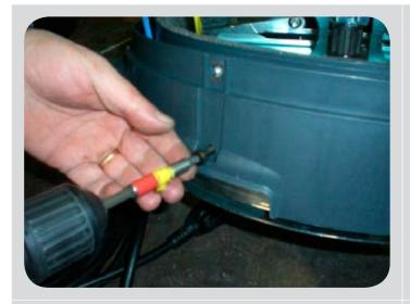
Remove the base of the motor cover, unscrewing the 3 screws at the base.
