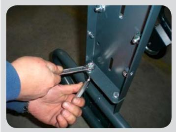
To remove and replace the whole upright, unscrew the 2 bolts holding it on the trolley.
