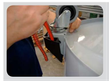
To remove and replace the container wheels, remove the plastic wheel guard using a suitable wrench.
