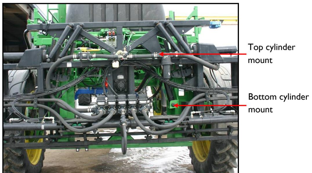
**Figure 14: Roll Cylinder Mounts**
