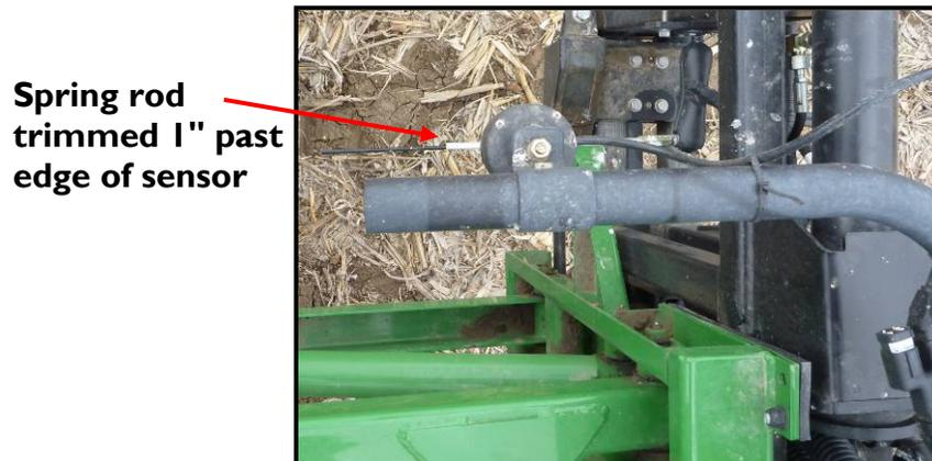
**Figure 39: Active Roll™ Sensor and Rod Alignment**
