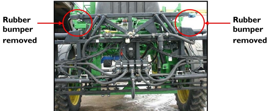
Figure 17: Rubber Bumpers Removed
