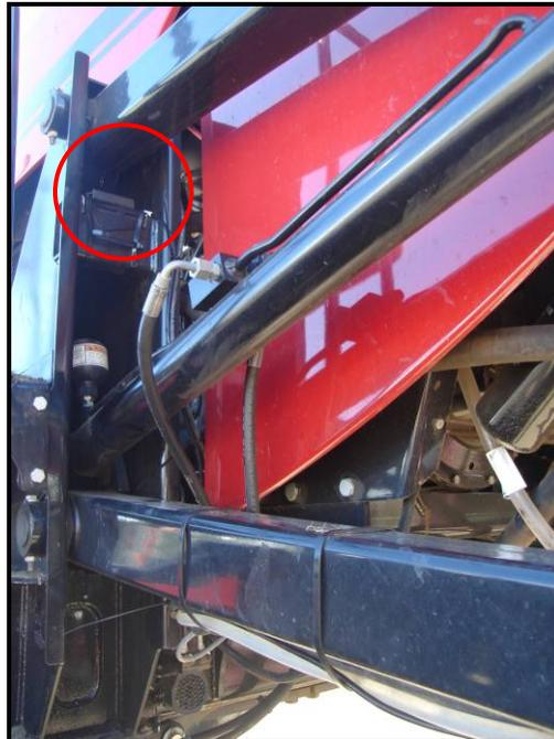
**Figure 36: Example of Reference Frame Roll Sensor Mounting**
