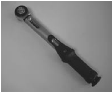
Torque wrench, measurement range 10 Nm to 50 Nm
