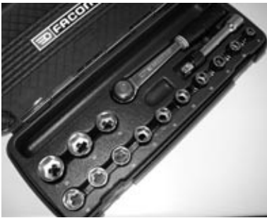
Reversible ratchet handle wrench and sockets, sizes 8 mm to 19 mm
