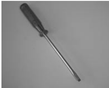
Screw driver, blade width 2.5 mm
