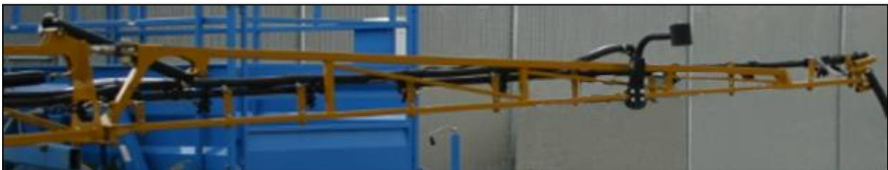
**Figure 23: Example Mounting of Outer Wing Sensor Bracket**
