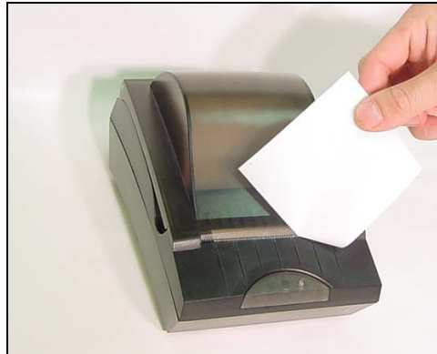
Figure 7: Tear off excess - SP
