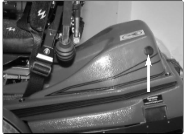
2. Unscrew the adjustment device with the enclosed special key.
