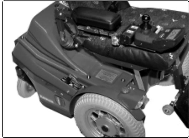
4. Open the electronics box and disconnect the contact for the rear light.
