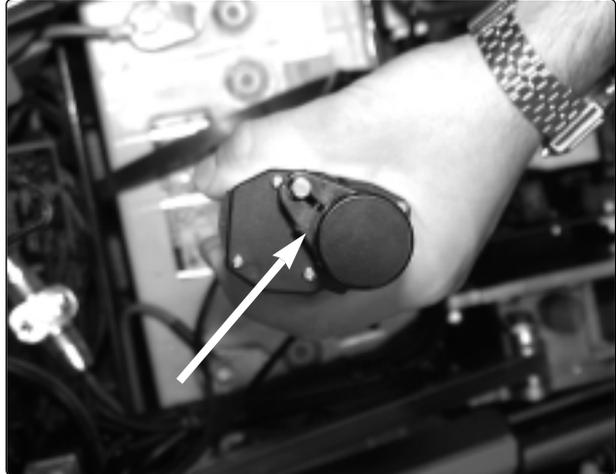
8. Loosen the screws which hold the limit switch. Pull away the adjustment device.
