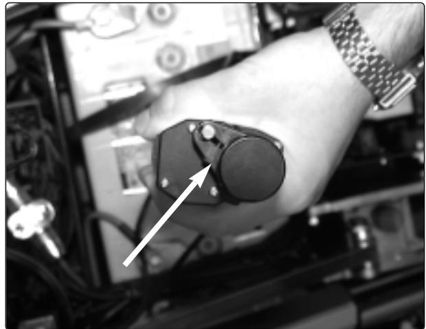
3. Tighten the front screw of the adjustment device.
