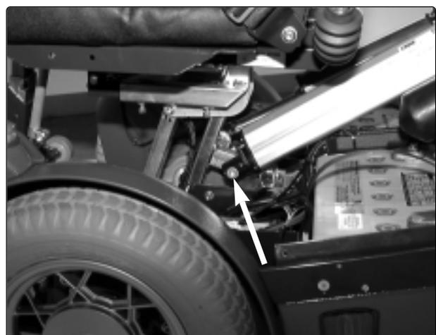
7. Remove the clamping ring of the limit switch.
