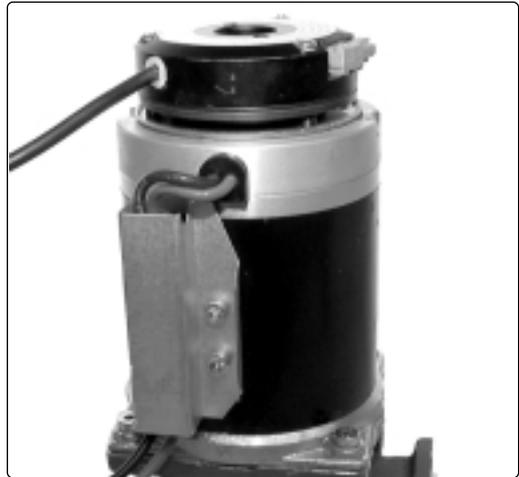
3. Remove the magnetic brake.
