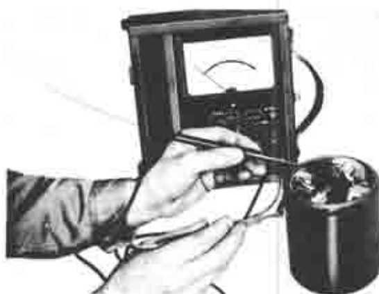
Fig. 5-27 Checking of field coil
