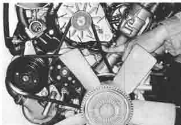
Fig. 1A-58 Checking of deflection
