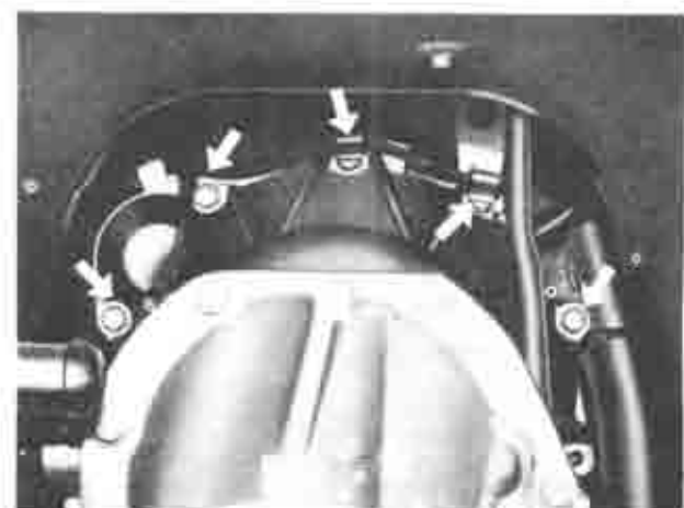
Fig. 2-10 Bolts on engine & converter housing
