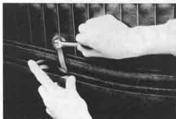
Fig. 14-19 Removing of regulator handle
