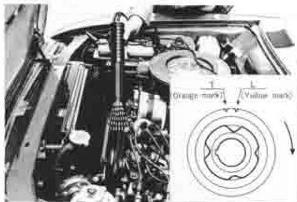
Fig. 1A-64 Adjusting of ignition timing
