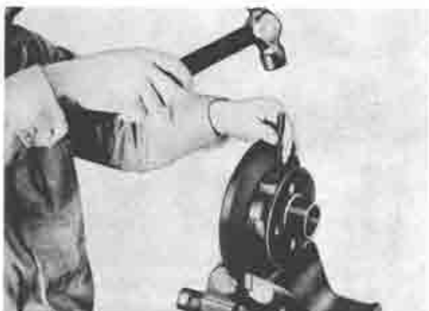
Fig. 11-24 Applying of identification marks
