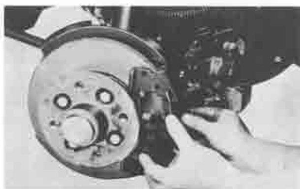
Fig. 11-17 Removing of caliper
