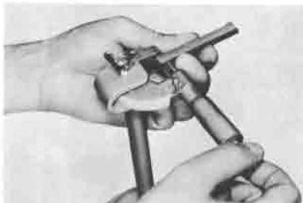
Fig. 1-60 Measuring apex seal height
