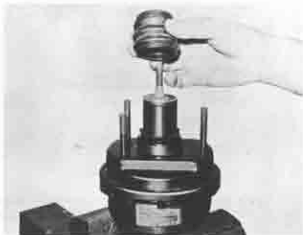
Fig. 11-7 Removing of boot
