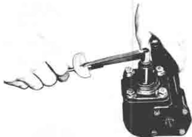
Fig. 10-11 Checking of preload
