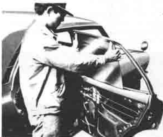
Fig. 14-26 Removing of glass
