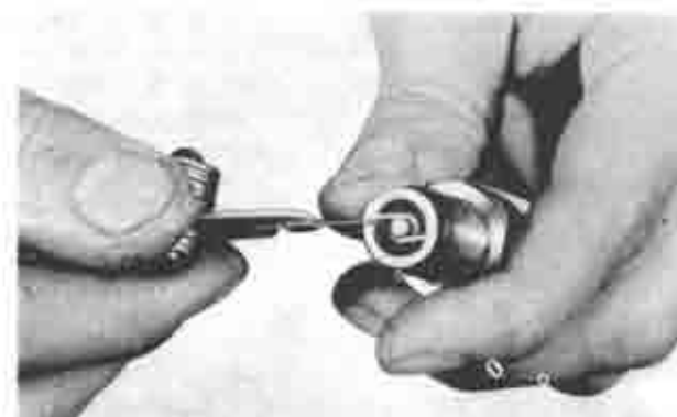
Fig. 5-2 Adjusting spark plug gap
