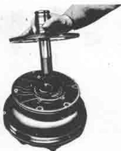
Fig. 2-40 Assembling oil pump
