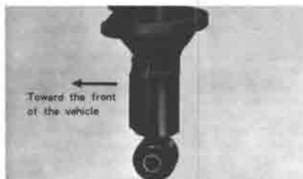
Fig. 13-30 Lower of rear shock absorber
