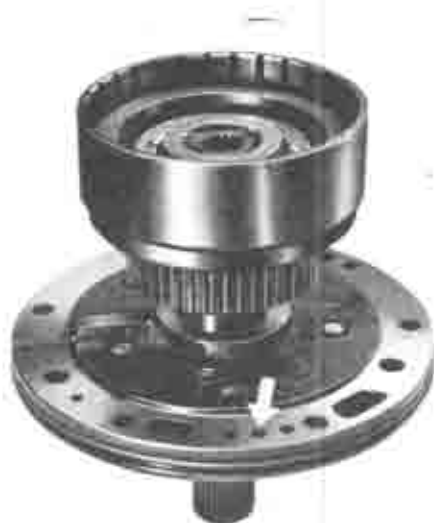
Fig. 2-25 Rear clutch testing hole
