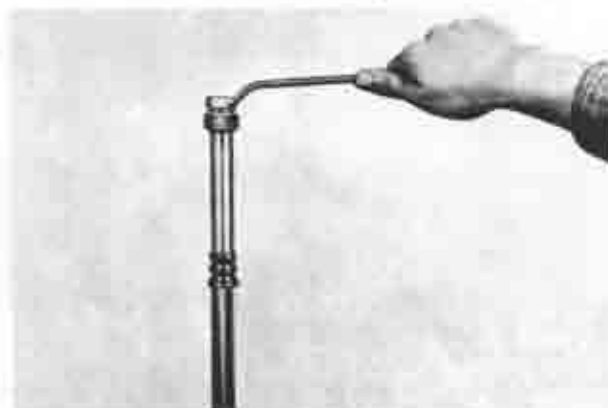
Fig. 13-10 Removing of piston nut
