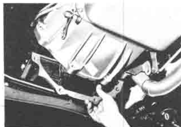
Fig. 2-8 Removing under cover
