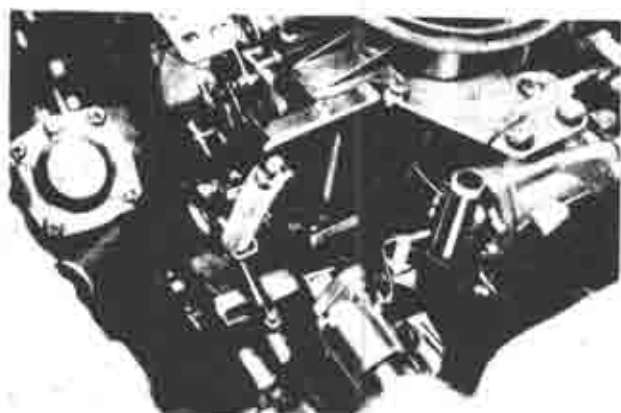
Fig. 1A-24 Anti-afterburn valve
