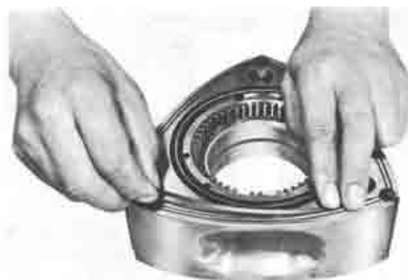
Fig. 1-77 Fitting side seal
