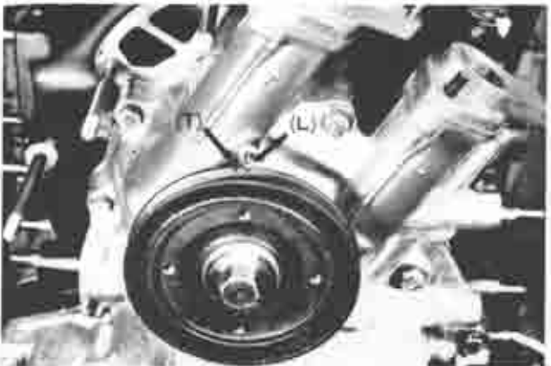
Fig. 1-101 Aligning for top dead center
