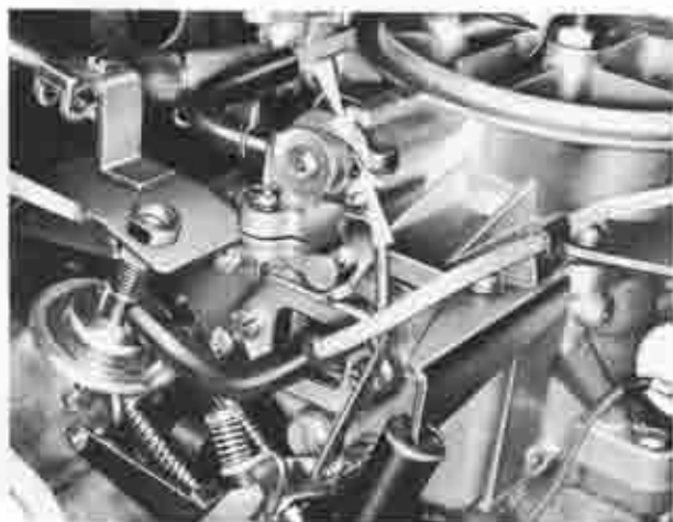
Fig. 1A-63 Adjusting of return spring
