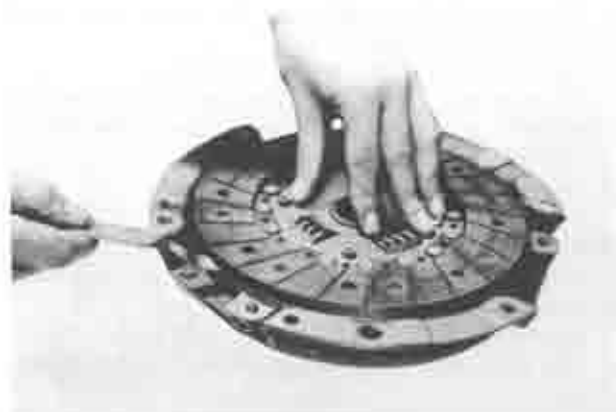
Fig. 6-4 Checking clutch disk
