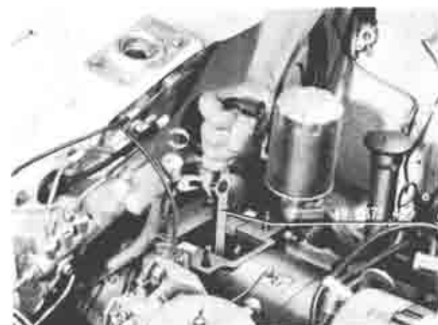
Fig. 2-9 Loosening bolts on the converter
