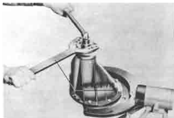
Fig. 9-13 Removing of drive pinion nut
