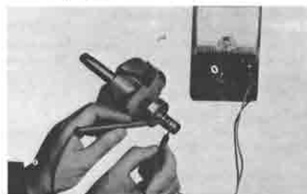
Fig. 5-12 Checking of rotor for open
