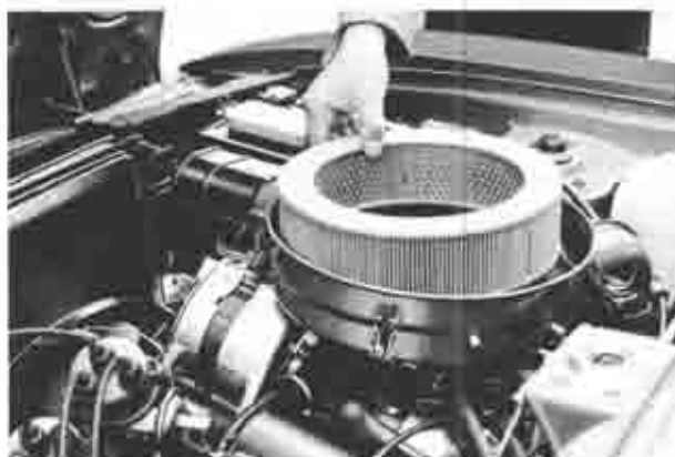
Fig. 1A-59 Replacing of element
