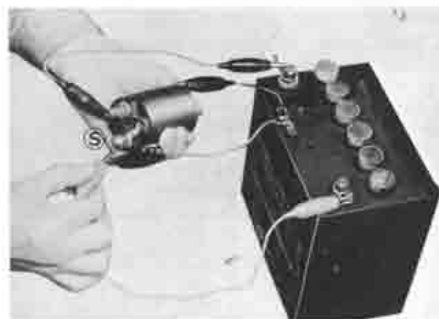
Fig. 5-30 Holding coil test
