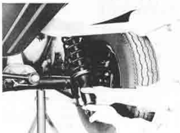
Fig. 13-27 Removing of rear shock absorber
