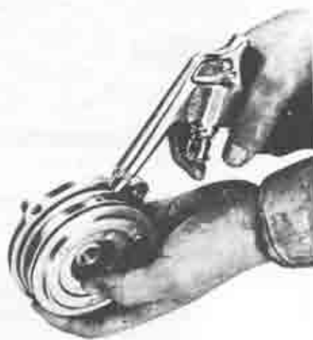
Fig. 2-31 Blowing out piston
