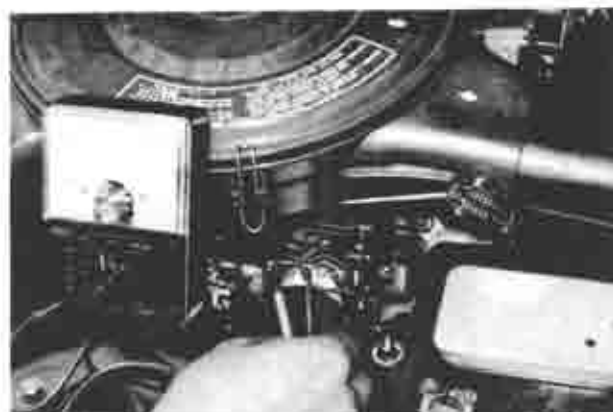
Fig. 1A-59 Checking of idle switch
