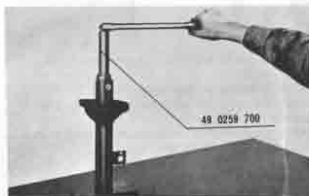
Fig. 13-22 Tightening of cap nut
