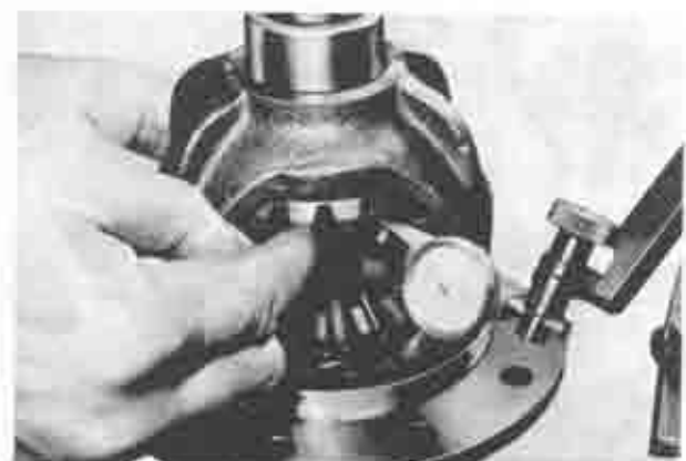
Fig. 9-24 Checking of backlash
