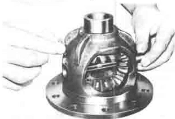
Fig. 9-25 Installing of lock pin
