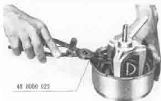
Fig. 2-19 Removing snap ring
