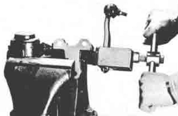
Fig. 10-4 Removing of pitman arm
