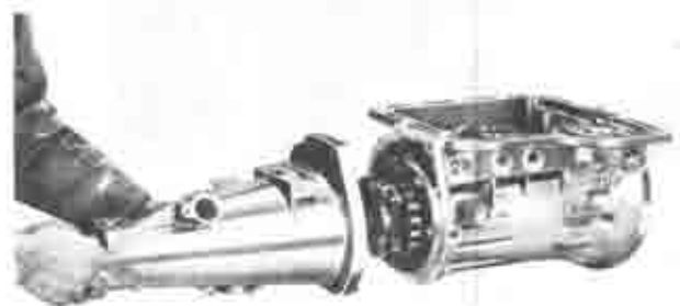
Fig. 2-17 Removing extension housing
