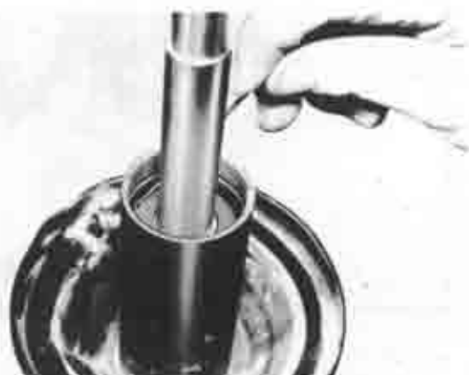
Fig. 13-9 Removing of "O" ring
