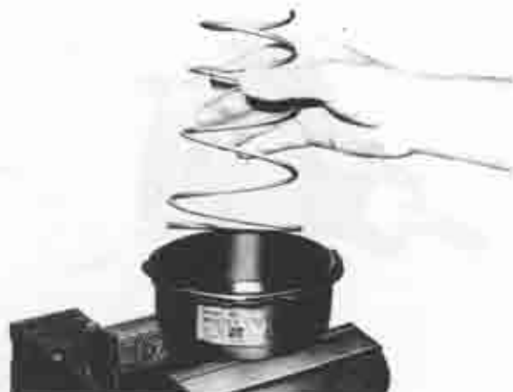
Fig. 11-9 Removing of return spring
