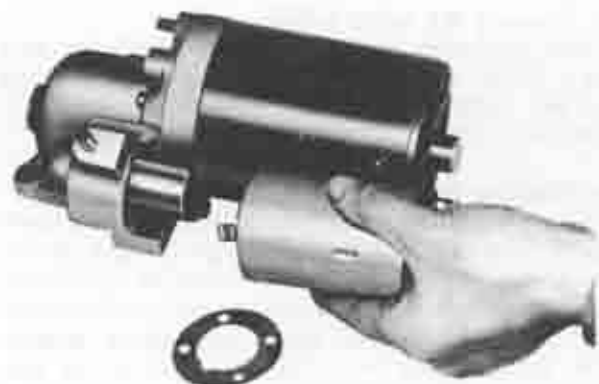
Fig. 5-21 Removing of magnetic switch
