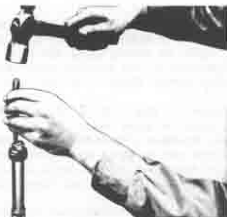
Fig. 13-17 Applying of punch
