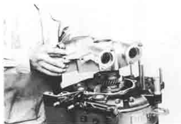
Fig. 1-96 Installing front cover
