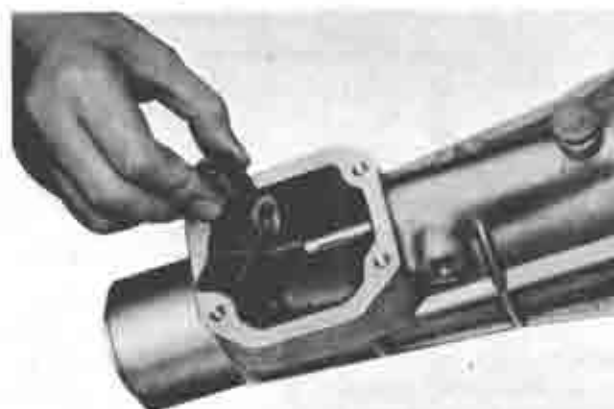
Fig. 7-14 Installing control lever end
