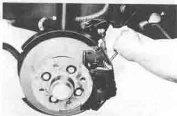
Fig. 11-16 Removing of stop plates
