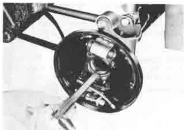
Fig. 9-5 Measuring of depth
