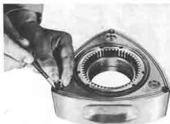
Fig. 1-76 Fitting corner seal
