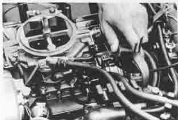
Fig. 1A-63 Checking of air supply valve
