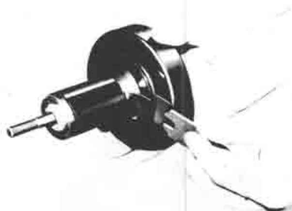
Fig. 11-12 Removing of retainer key
