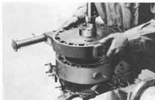
Fig. 1-86 Installing intermediate housing
