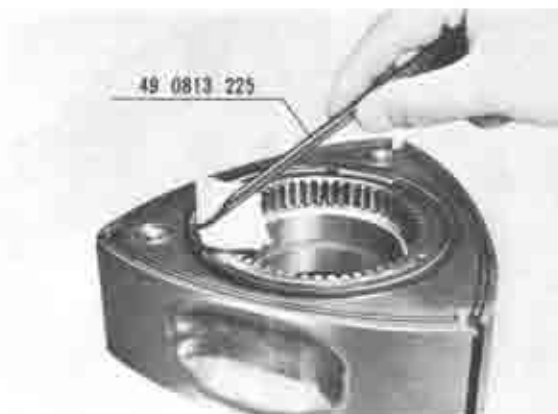
Fig. 1-45 Removing oil seals
