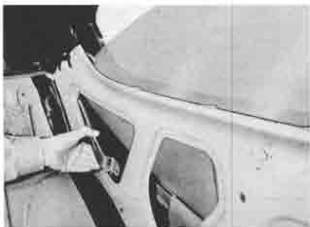
Fig. 14-31 Removing of glass guide
