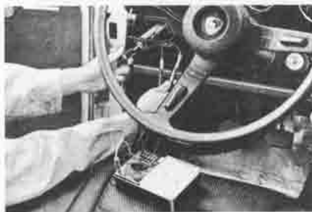
Fig. 1A-62 Checking of choke switch
