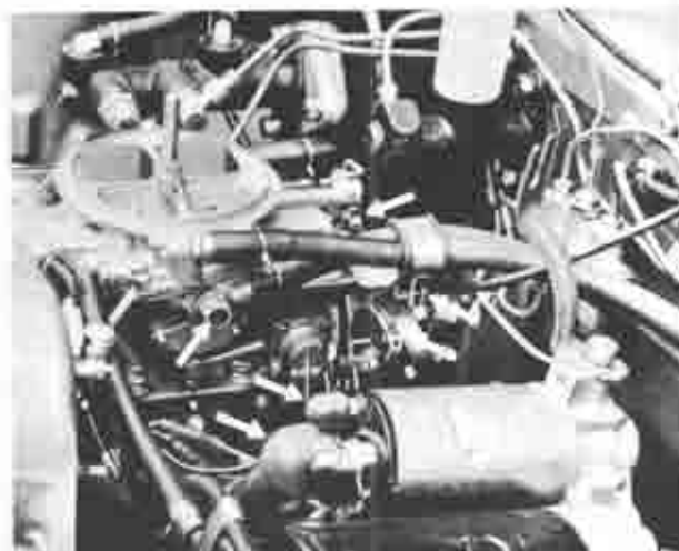
Fig. 1-5 Disconnecting pipes and cables
