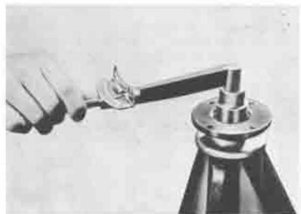
Fig. 9-21 Checking of preload
