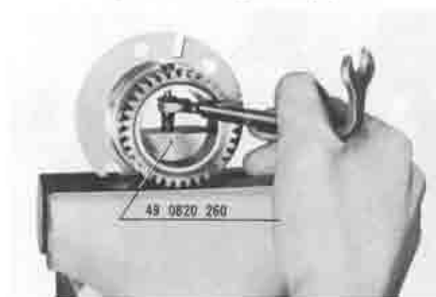
Fig. 1-33 Removing lock pin
