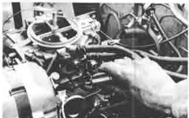
Fig. 1A-74 Adjusting of idle mixture
