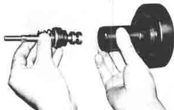
Fig. 11-13 Removing of valve rod and plunger
