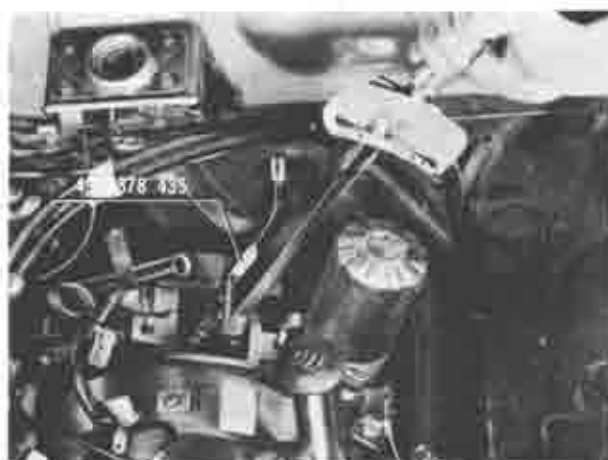
Fig. 2-53 Measuring tightening torque
