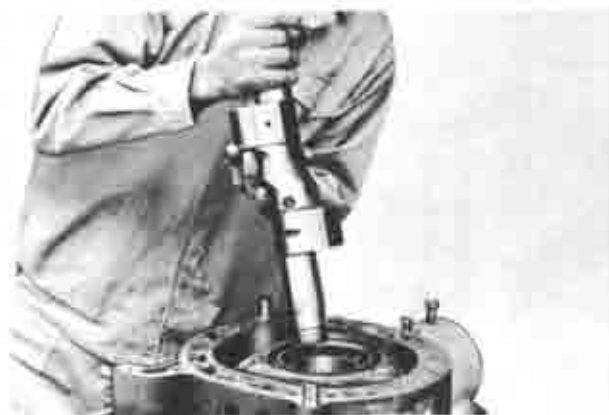
Fig. 1-84 Installing eccentric shaft
