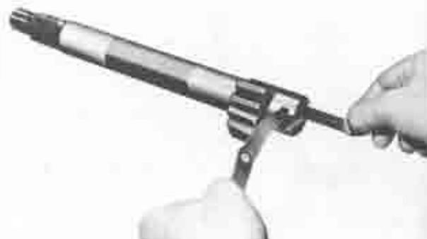
Fig. 10-7 Checking of end clearance
