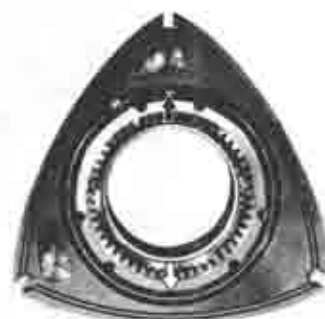
Fig. 1-74 Position of spring gap
