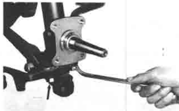
Fig. 13-4 Removing of two bolts
