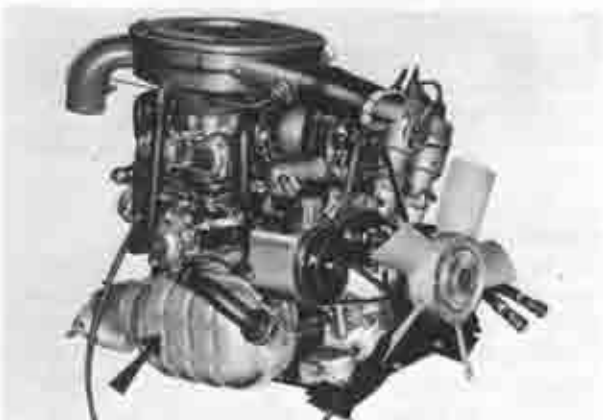
Fig. 1A-8 Thermal reactor
