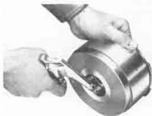
Fig. 2-20 Blowing out piston
