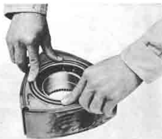
Fig. 1-75 Installing oil seal
