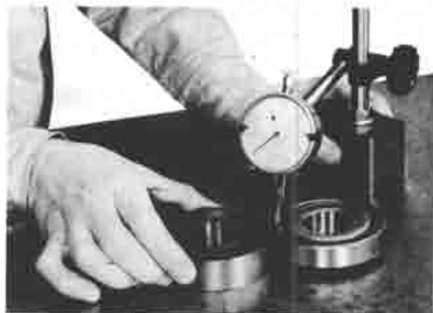
Fig. 9-18 Measuring of bearing height
