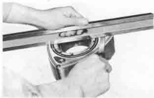
Fig. 1-48 Inspection land protrusion.
