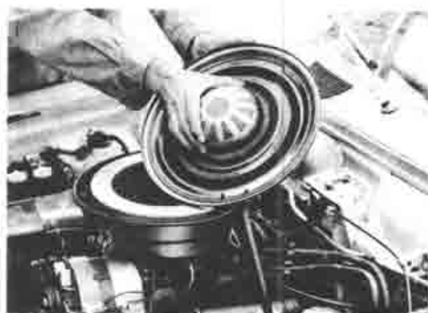
Fig. 1A-66 Removing of charcoal filter
