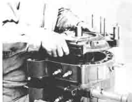
Fig. 1-19 Removing front housing
