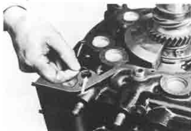
Fig. 1-95 Fitting "O" ring
