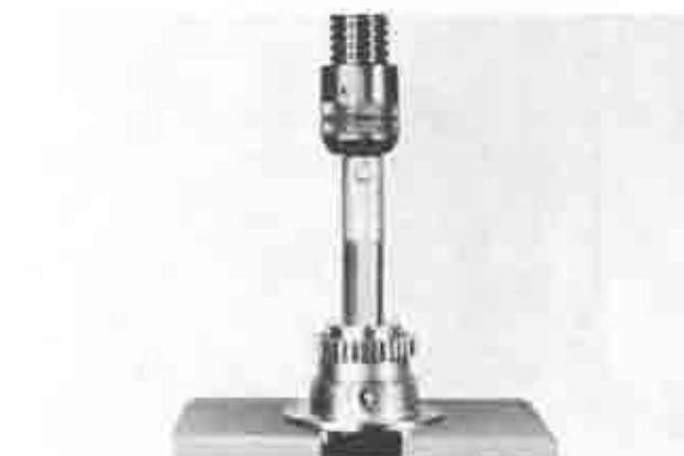
Fig. 1-34 Removing main bearing
