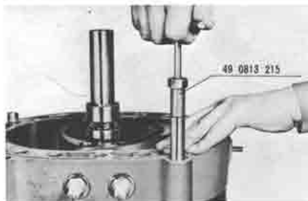
Fig. 1-20 Pulling tubular dowels
