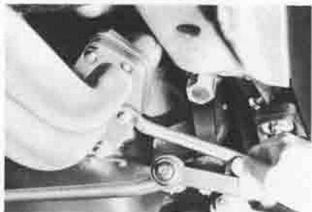
Fig. 1-8 Disconnecting exhaust pipe
