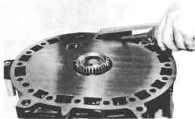
Fig. 1-28 Cleaning front housing
