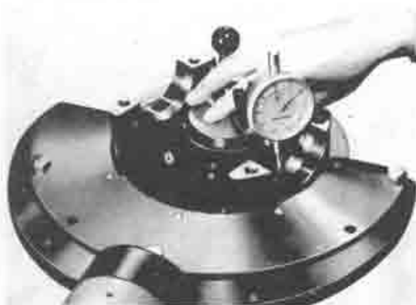
Fig. 9-17 Measuring of pinion height
