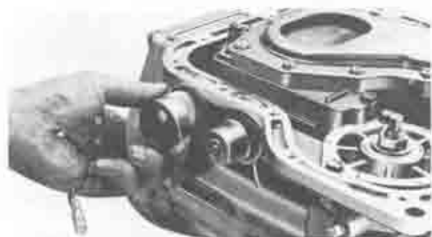
Fig. 2-12 Removing downshift solenoid
