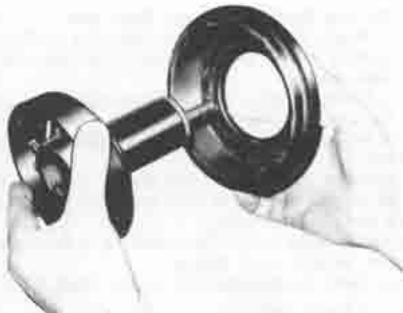
Fig. 11-11 Removing of diaphragm
