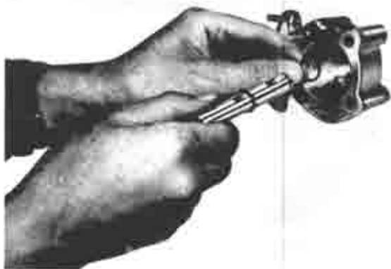
Fig. 2-7 Assembling oil pump
