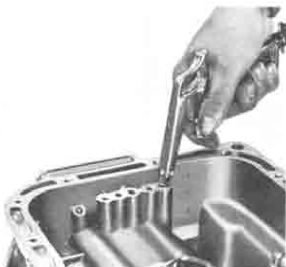
Fig. 2-27 Blowing out piston
