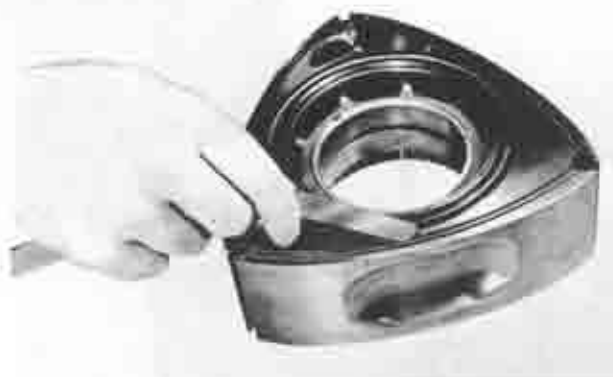
Fig. 1-63 Checking side seal gap
