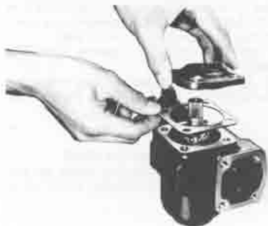
Fig. 10-6 Installing of end cover and shim
