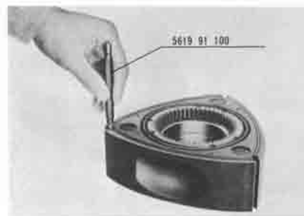
Fig. 1-65 Checking gap of corner seal and groove
