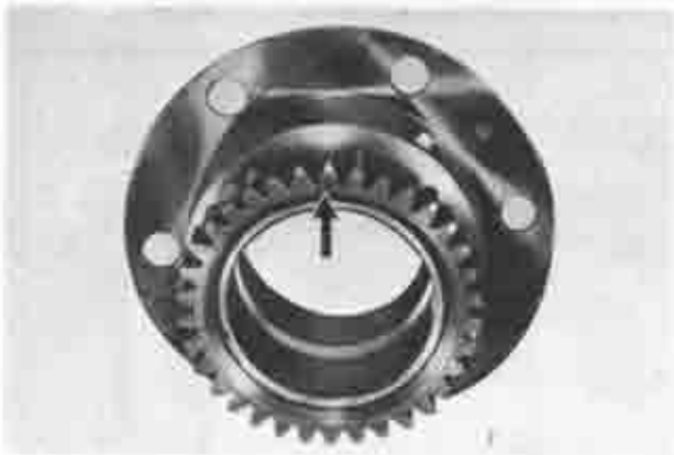
Fig. 1-58 Mark of stationary gear
