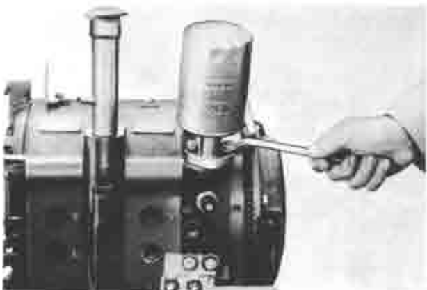
Fig. 1-100 Installing oil filter
