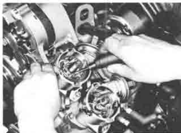
Fig. 1A-67 Adjusting of point gap
