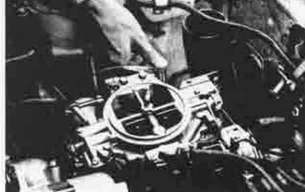
Fig. 1A-57 Checking of anti-afterburn valve
