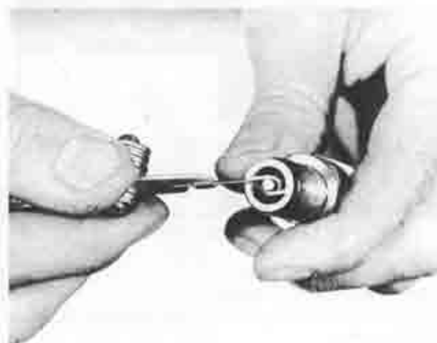
Fig. 1A-71 Adjusting of electrode gap
