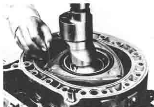
Fig. 1-85 Fitting apex seal spring
