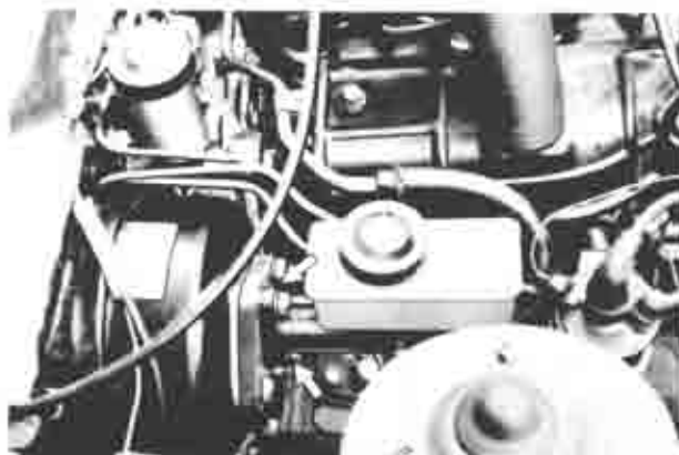
Fig. 11-1 Removing of Brake Master Cylinder
