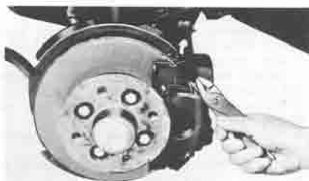
Fig. 11-15 Removing of fastening clips
