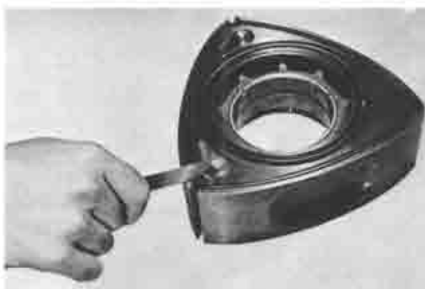
Fig. 1-68 Checking gap of corner seal and side seal
