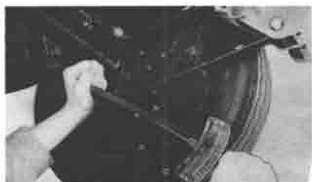
Fig. 13-33 Tightening of links
