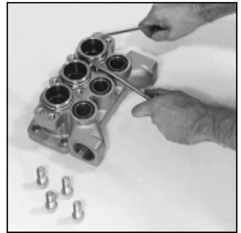
3520, 3521, 3527 Removal of V-Packing Cylinder
