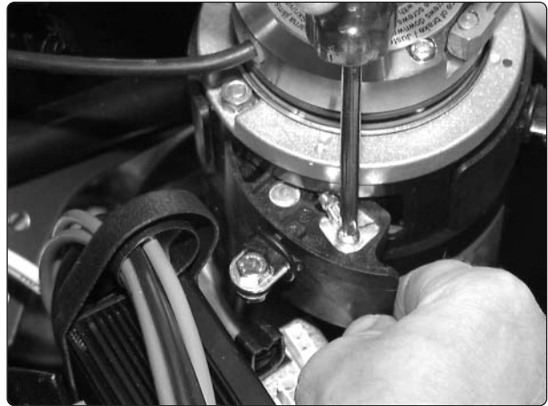
Loosen the cable connection
