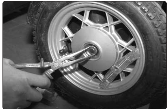
Thread off the axle nut
