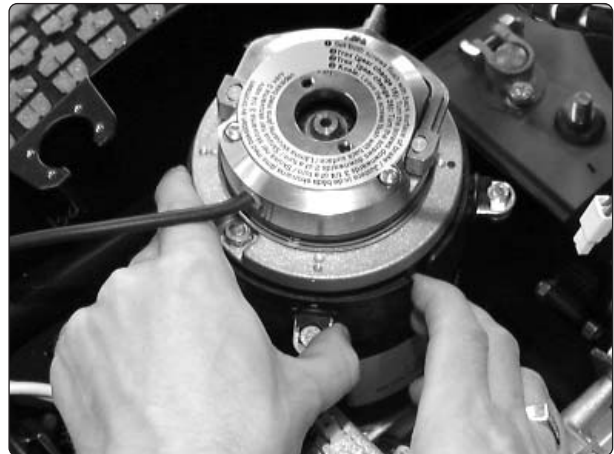
Removing a brush holder
