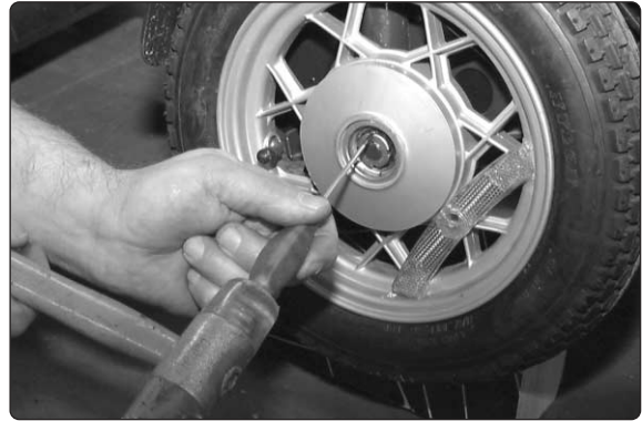
Release the axle nut
