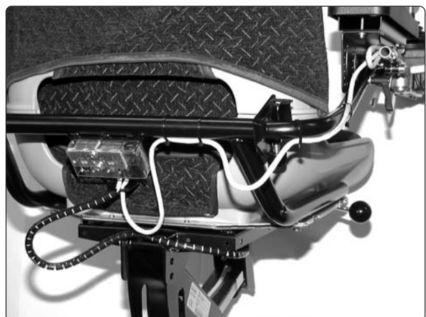
Cable laying behind the seat (seen from the rear)
