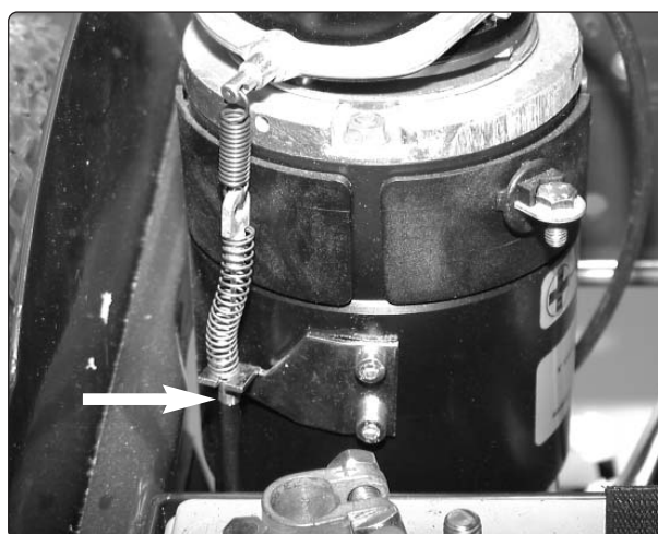
Brake release wire
