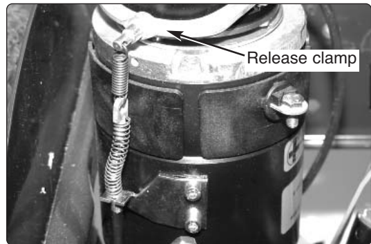
Fastening the wire at the brake
