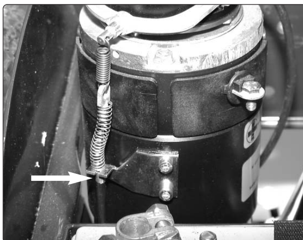
Brake release wire
