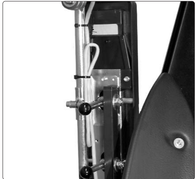
Cable laying under the CII/T arm rest (seen from beneath)
