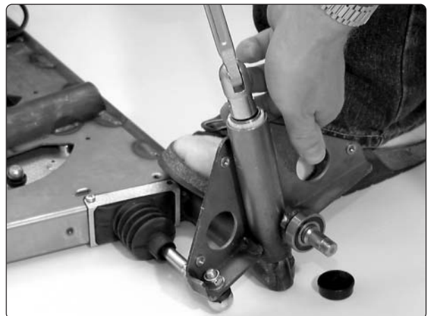
Screw the ball bearing back
