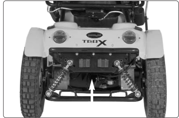
Location of the fuses
