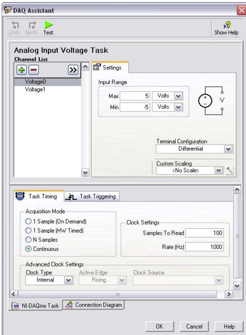
**Figure 9.** VI Logger analog input voltage task menu
