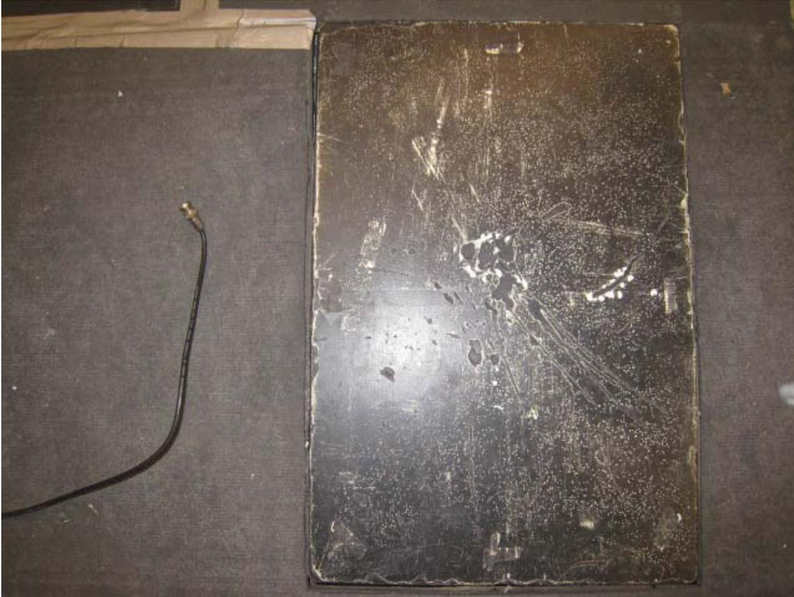
**Figure 5.** Kistler force platform with  $F_z$  output channel
