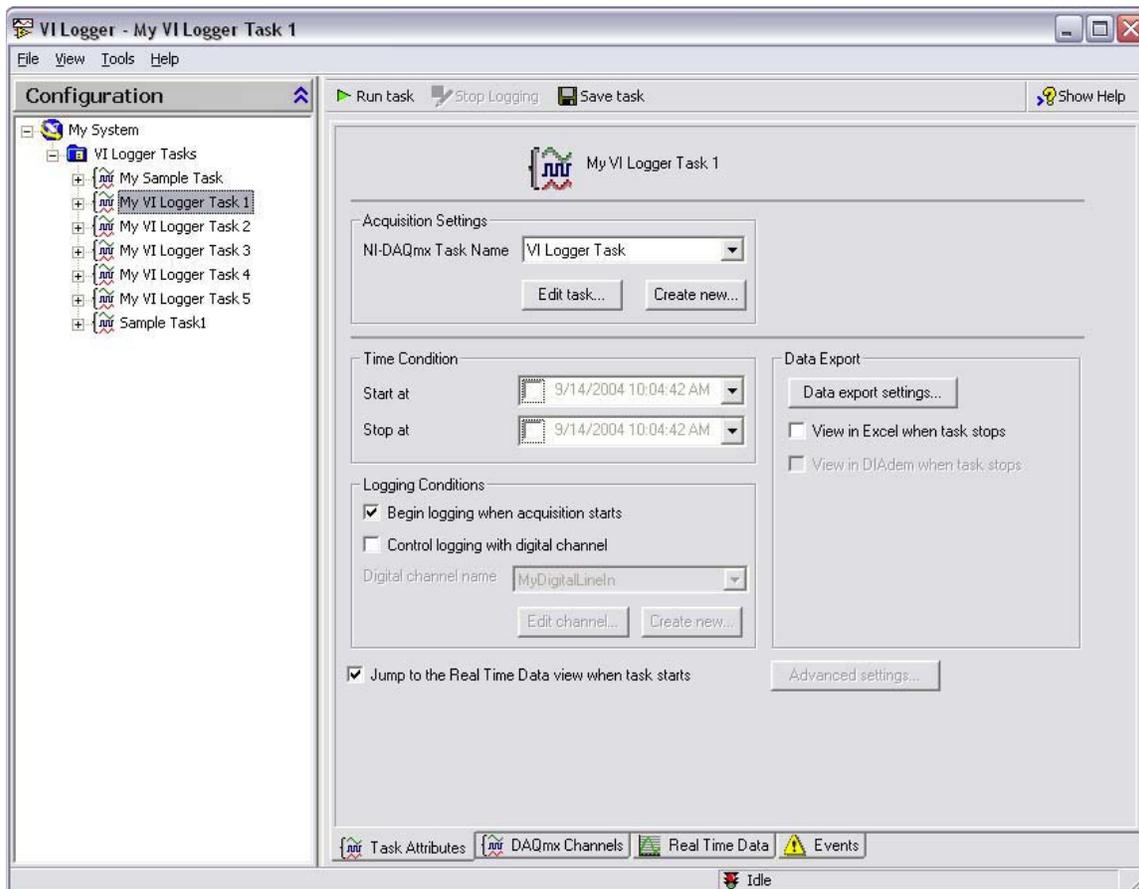
**Figure 4.** VI Logger configuration menu
