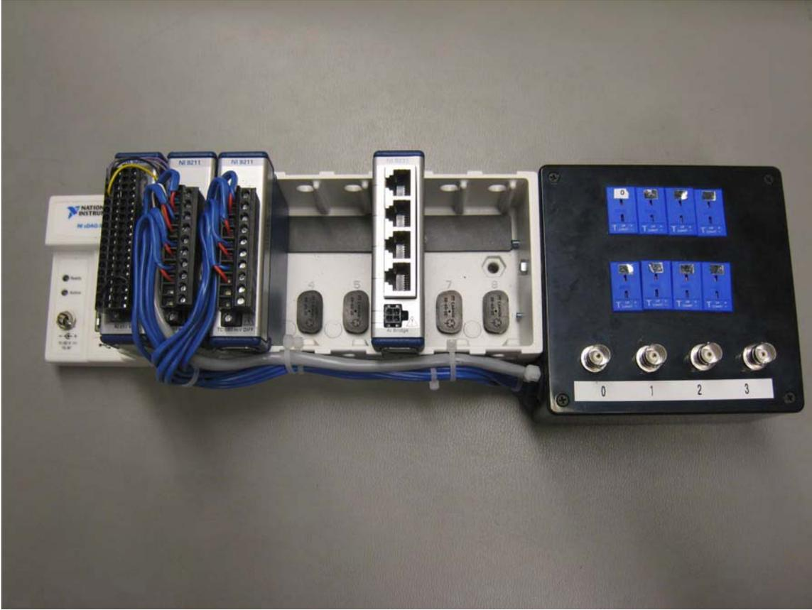
**Figure 7.** NI-DAQmx chassis with several modules. Only channel 6 (middle) is needed.
