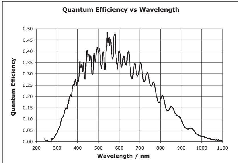
Figure 4.1: Spectral response of the A1024B CMOS sensor
