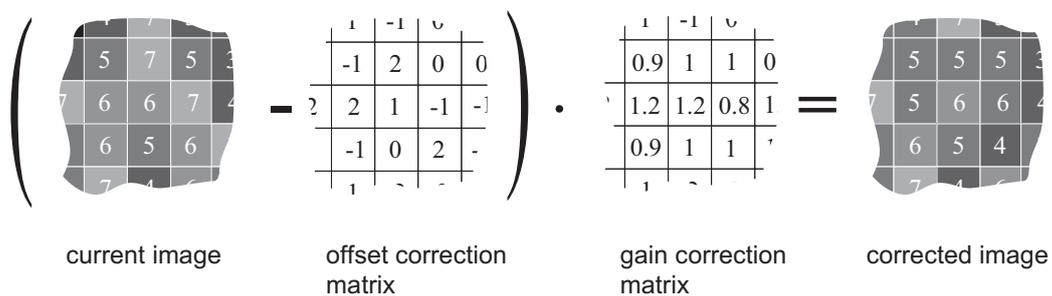
Figure 5.16: Schematic presentation of the corrected image using gain correction algorithm
