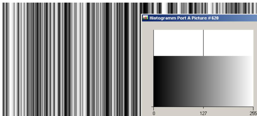
Figure 5.9: LFSR test pattern received at the frame grabber and typical histogram for error-free data transmission
