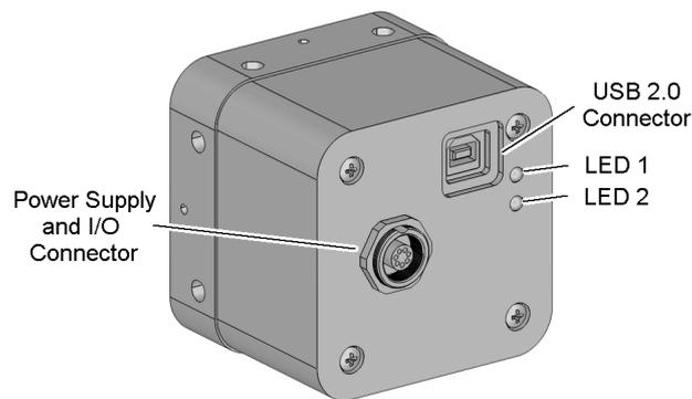
Figure 6.4: Rear view of the USB 2.0 cameras
