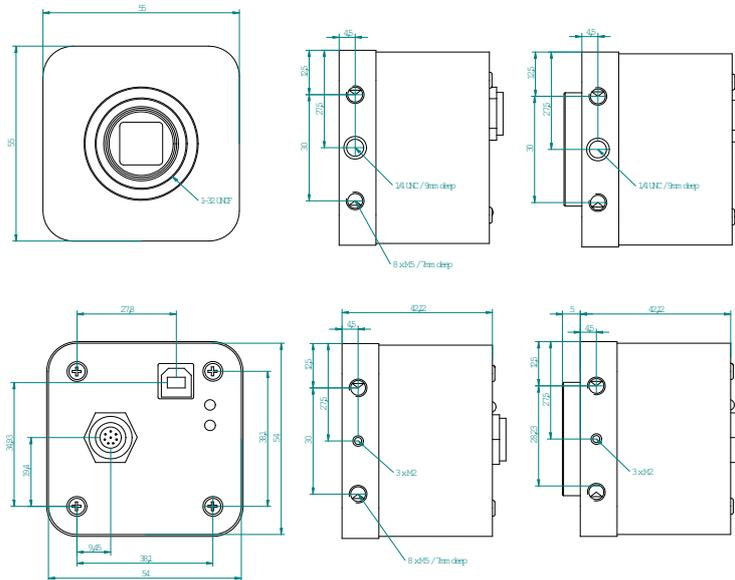
Figure 9.3: Mechanical dimensions of the USB 2.0 model, displayed without and with C-Mount adapter
