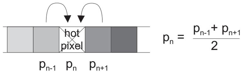
Figure 5.13: Hot pixel interpolation
