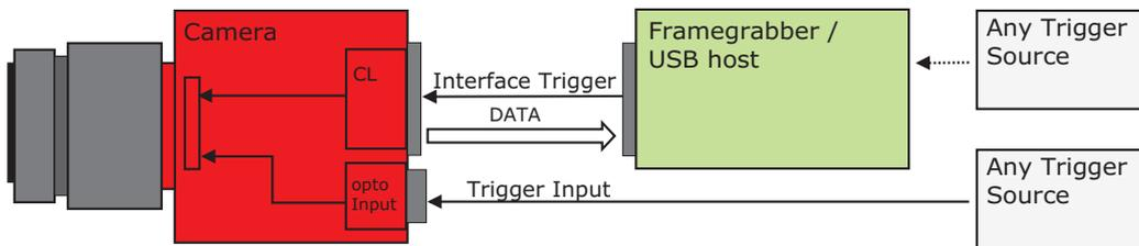
Figure 5.18: Trigger Inputs
