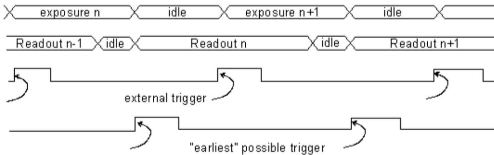
Figure 5.6: Timing in triggered simultaneous readout mode
