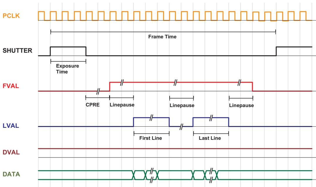
Figure 6.8: Timing diagram sequential readout mode
