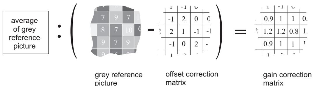
Figure 5.14: Schematic presentation of the gain correction algorithm
