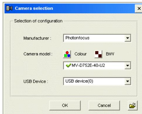
Figure 3.3: MicroDisplayUSB camera selection window
