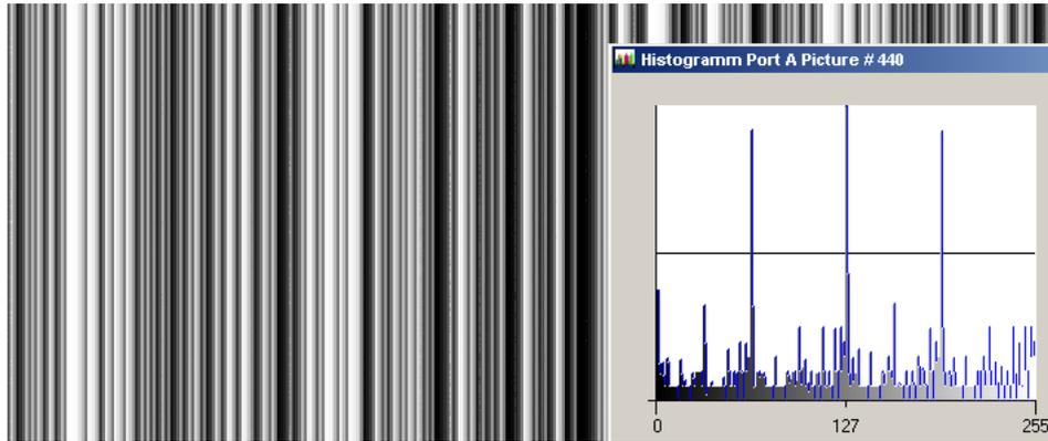
Figure 5.10: LFSR test pattern received at the frame grabber and histogram containing transmission errors
