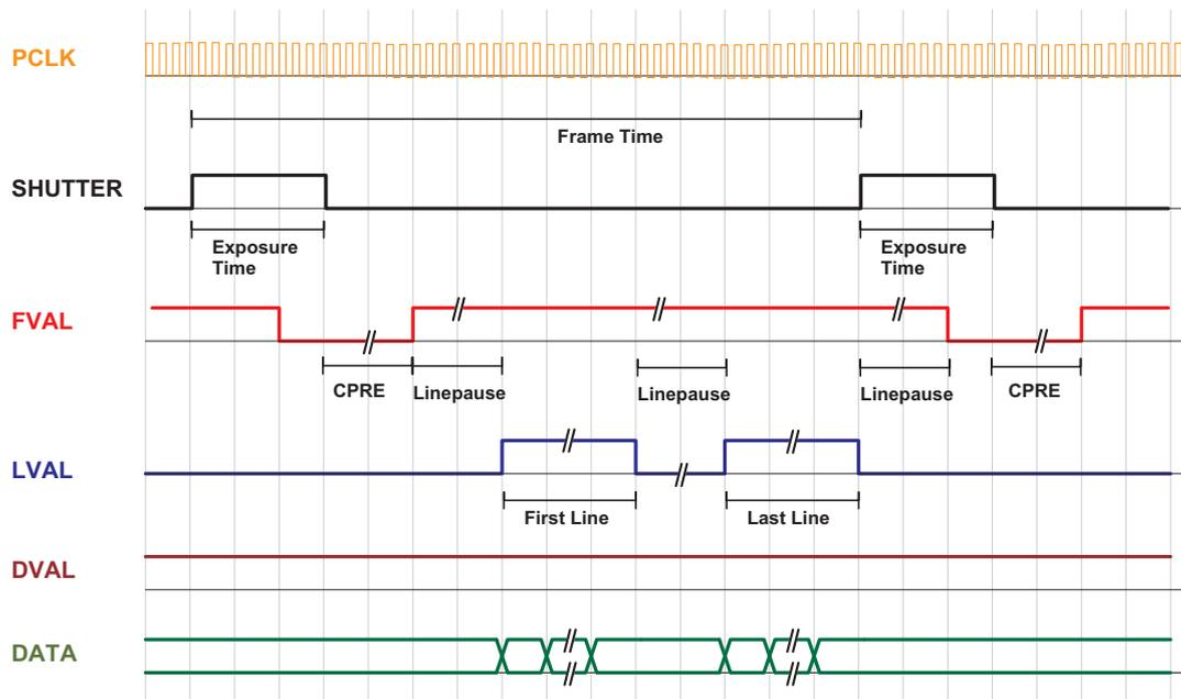
Figure 6.9: Timing diagram simultaneous readout mode (readout time > exposure time)
