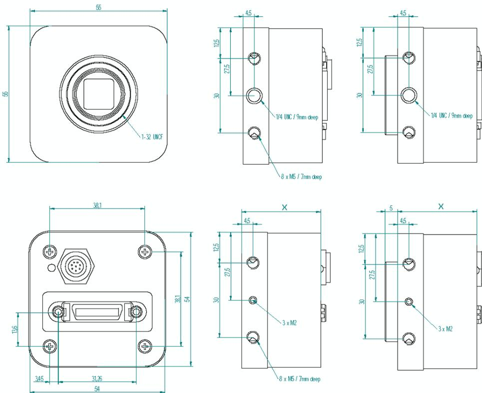
Figure 9.1: Mechanical dimensions of the CameraLink model, displayed without and with C-Mount adapter
