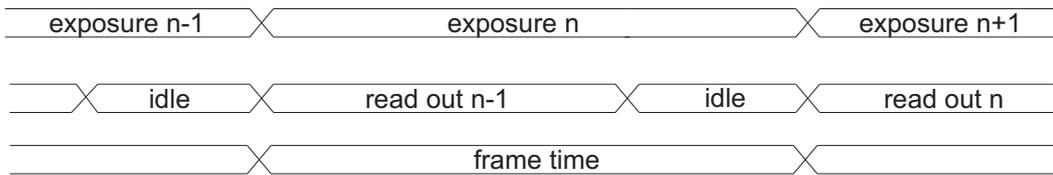
Figure 5.5: Timing in free-running simultaneous readout mode (readout time < exposure time)
