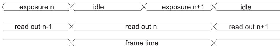
Figure 5.4: Timing in free-running simultaneous readout mode (readout time > exposure time)
