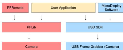
Figure 7.2: PFRemote and PFLib in context with the USB 2.0 frame grabber software
