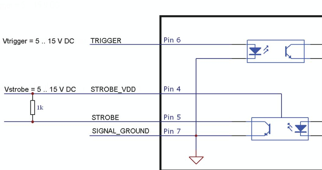
Figure 6.5: Circuit for the trigger input and strobe output signals
