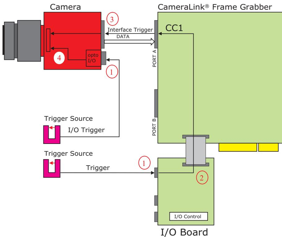
Figure 6.12: Trigger Delay visualisation from the trigger source to the camera
