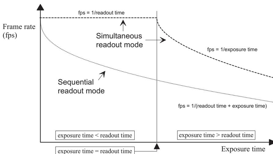
Figure 5.1: Frame rate in sequential readout mode and simultaneous readout mode
