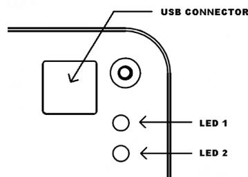
Figure 6.6: Position of the status indicator LEDs of the USB 2.0 cameras
