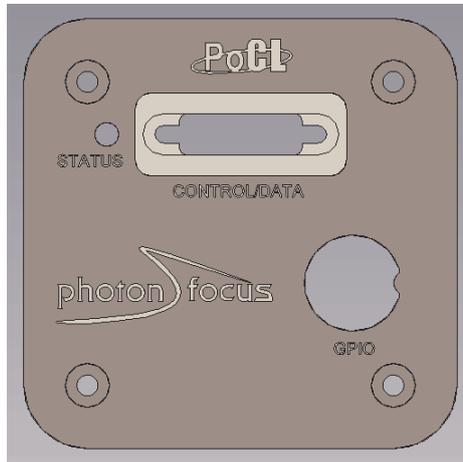
Figure 9.2: Drawing of the PoCL camera model rear view
