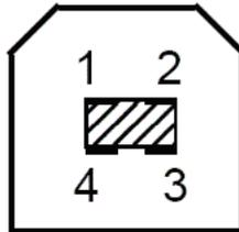
Figure A.7: USB type B connector (front view)
