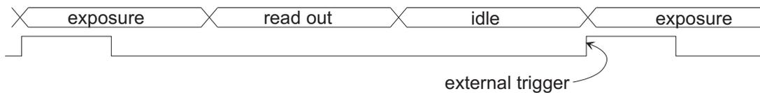
Figure 5.3: Timing in triggered sequential readout mode
