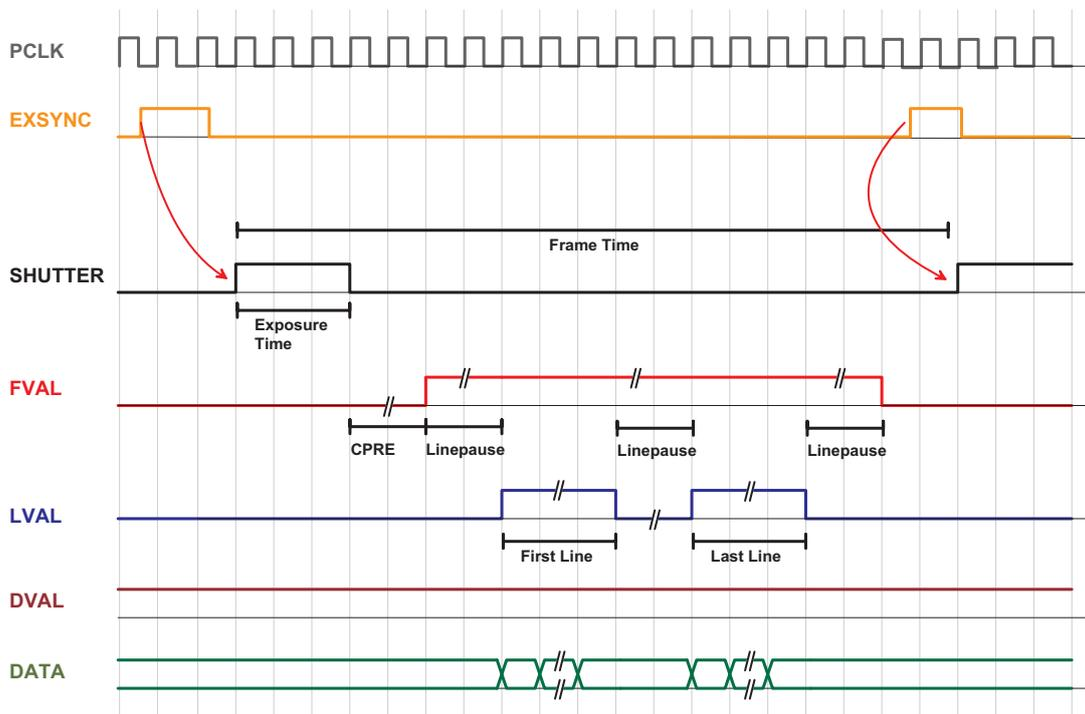
Figure 6.11: Trigger timing diagram for camera controlled exposure
