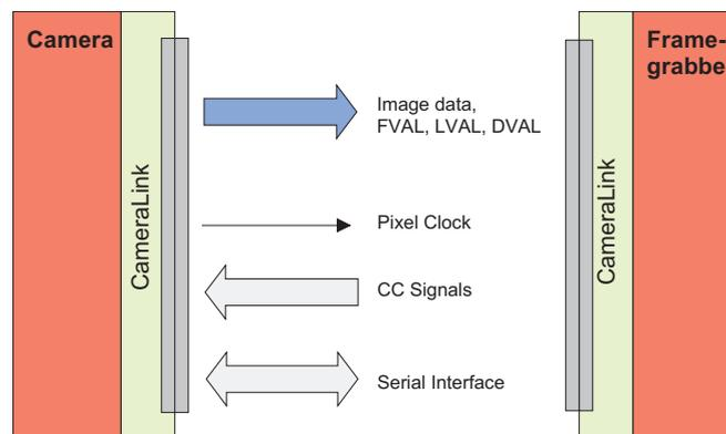
Figure 5.19: CameraLink serial interface for camera communication
