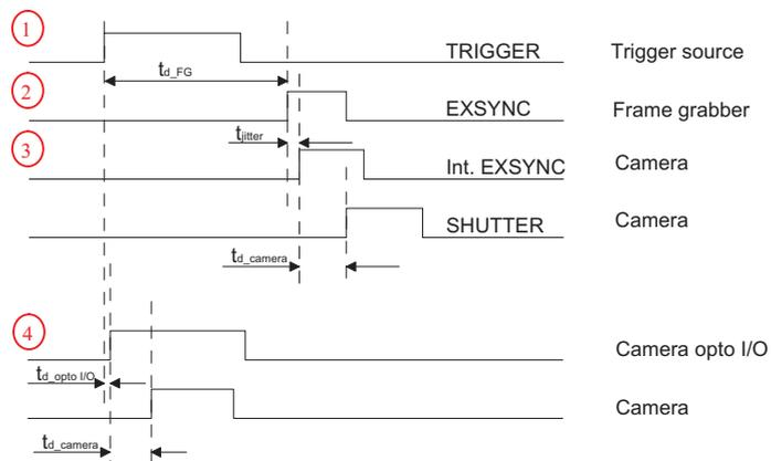
Figure 6.13: Timing Diagram for Trigger Delay
