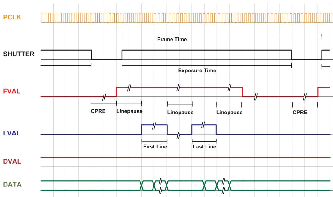
Figure 6.10: Timing diagram simultaneous readout mode (readout time < exposure time)
