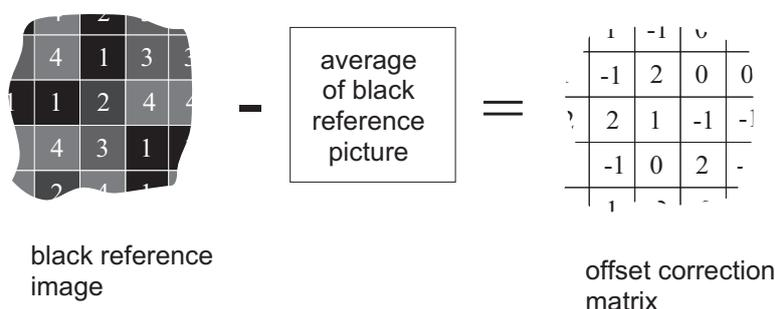
Figure 5.11: Schematic presentation of the offset correction algorithm
