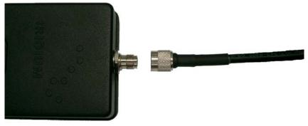
2. Plug the antenna cable into the antenna jack located on the top of the L-Band Transceiver
