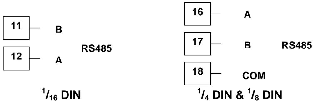
Figure 32. Option Slot A – RS485 Serial Communications Module
