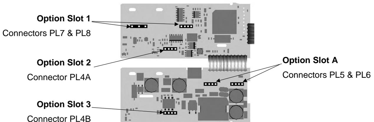
Figure 7. Option Module Connectors - 1/16 DIN Instruments
