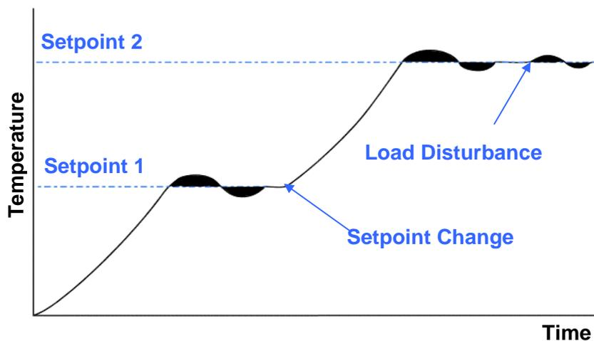
Figure 44. Self-Tune Operation
