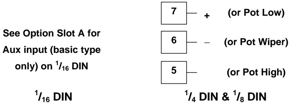
Figure 36. Option Slot B – Full Auxiliary Input Connections
