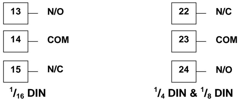
Figure 22. Option Slot 2 - Relay Module
