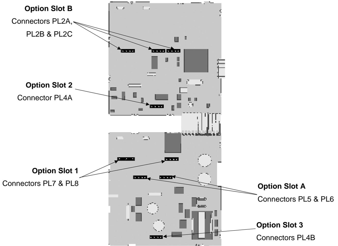
Figure 8. Option Module Connectors - 1/8 & 1/4 DIN Instruments
