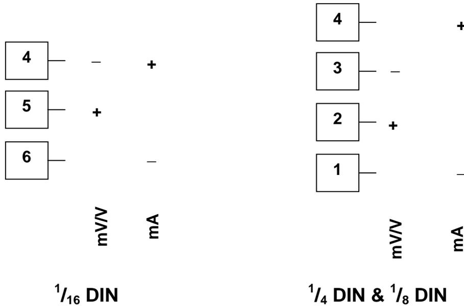
Figure 17. DC Volt, mV & mA Input Connections
