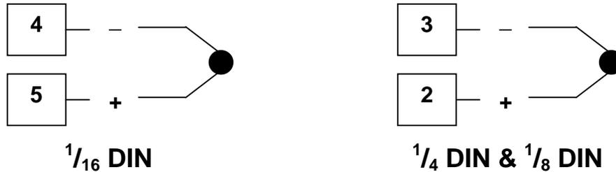
Figure 15. Thermocouple Input Connections
