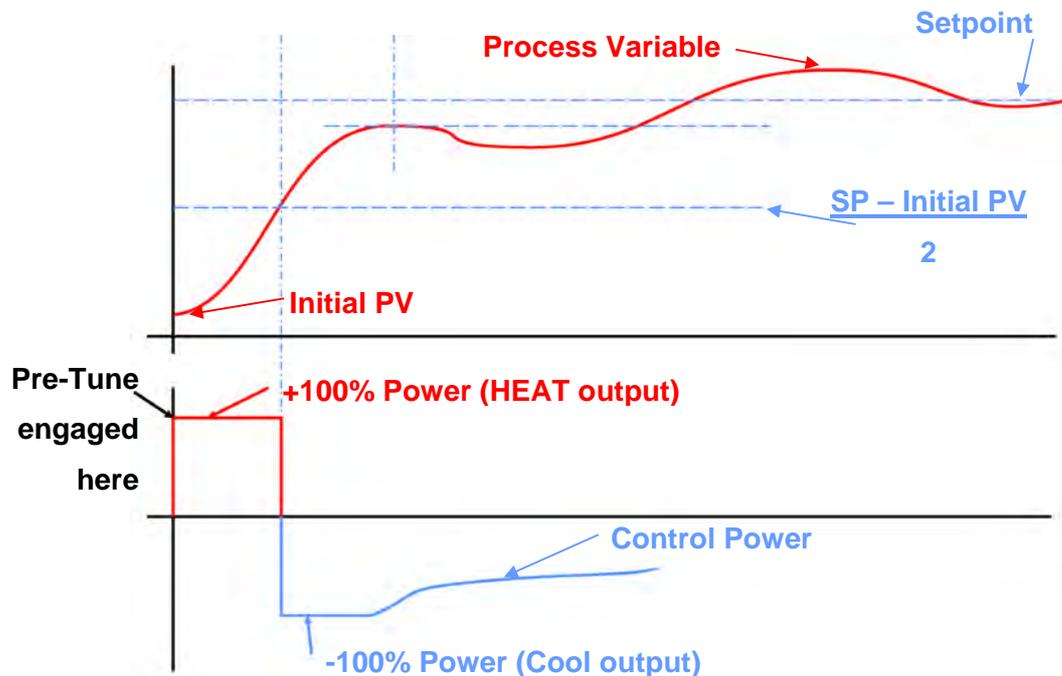
When Pre-Tune is completed, the PID control output power is applied using the calculated values. Pre-Tune limits the possibility of setpoint overshoot when the controller is new or the application has been changed. As a single-shot operation, it will automatically disengage once complete, but can be configured to run at every power up using the Auto Pre-Tune function.
