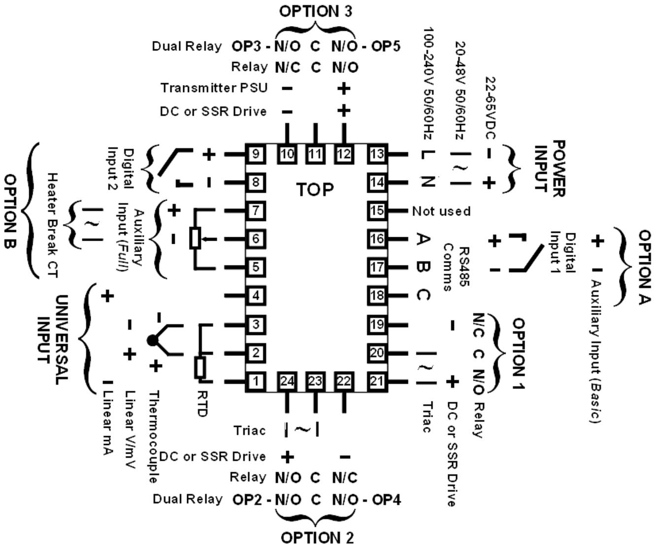
Figure 12. Rear terminals (1/4-DIN & 1/8-DIN Instruments)
