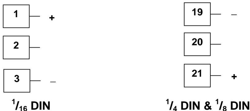
Figure 21. Option Slot 1 - Linear Voltage & mADC Module
