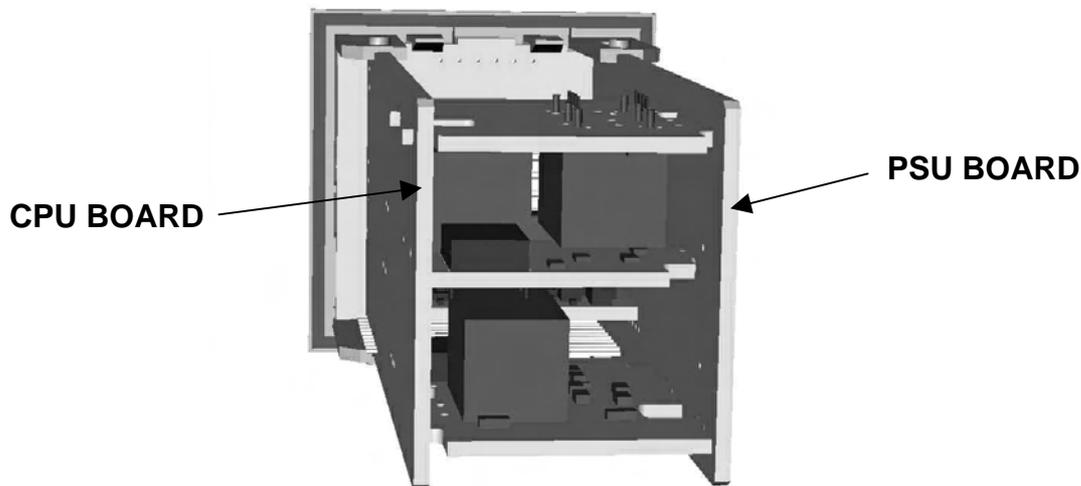
Figure 4. Typical rear view (uncased) & main board positions
