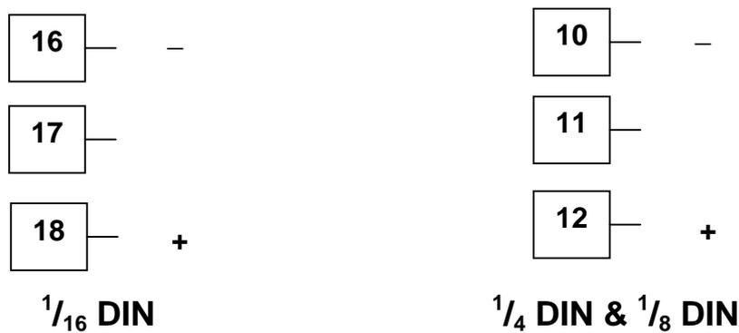
Figure 31. Option Slot 3 - Transmitter Power Supply Module
