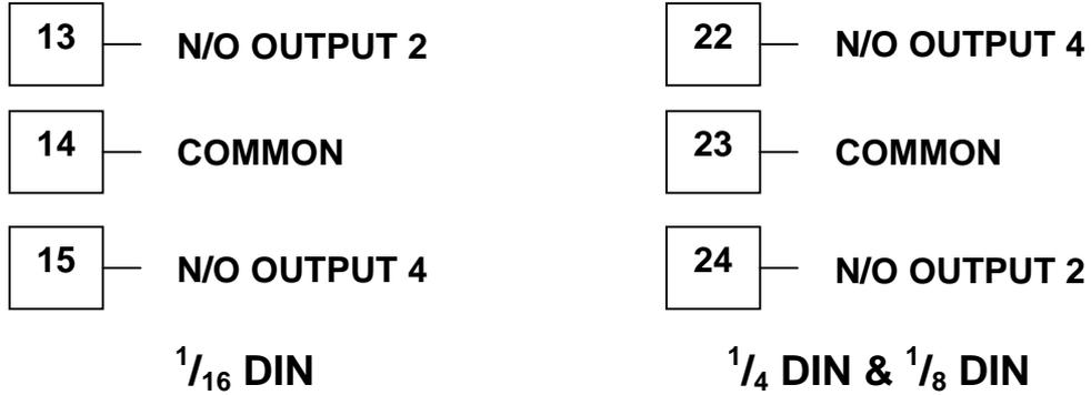
Figure 25. Option Slot 2 - Dual Relay Module
