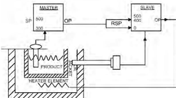
As the jacket temperature rises, the slave's heater output falls. The product temperature also rises at a rate dependant on the transfer lag between the jacket and product. This causes the master's PID output to decrease, reducing the 'jacket' setpoint on the slave, effectively reducing the output to the heater. This continues until the system becomes balanced.
