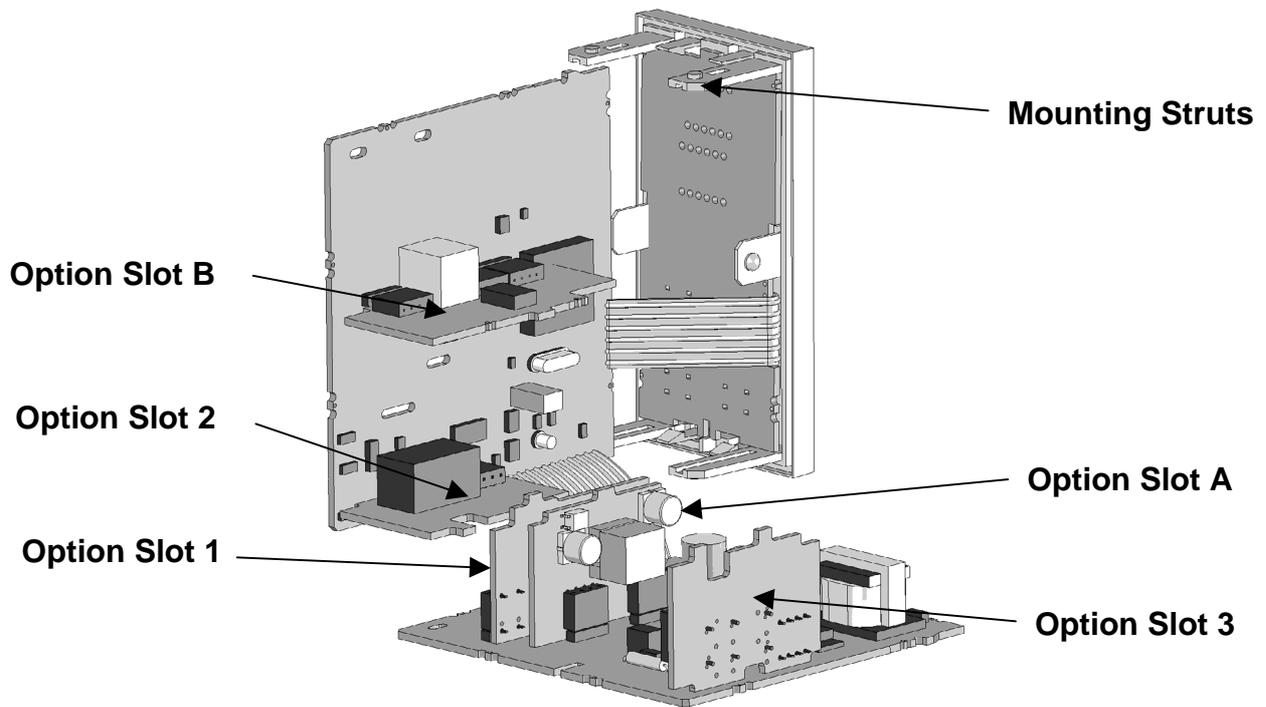
Figure 6. Location of Option Modules - 1/8 & 1/4 DIN Instruments
