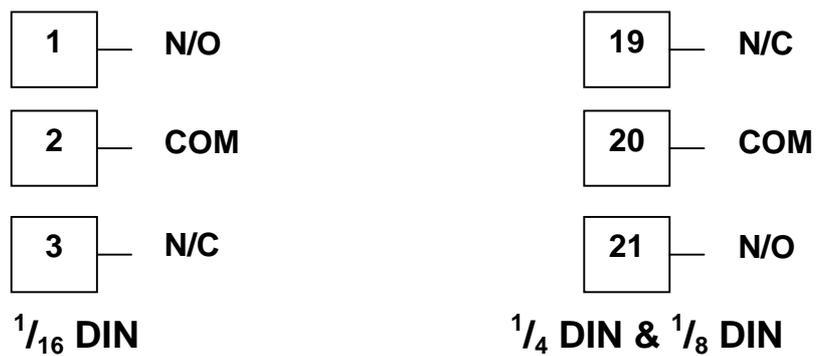
Figure 18. Option Slot 1 – Relay Module
