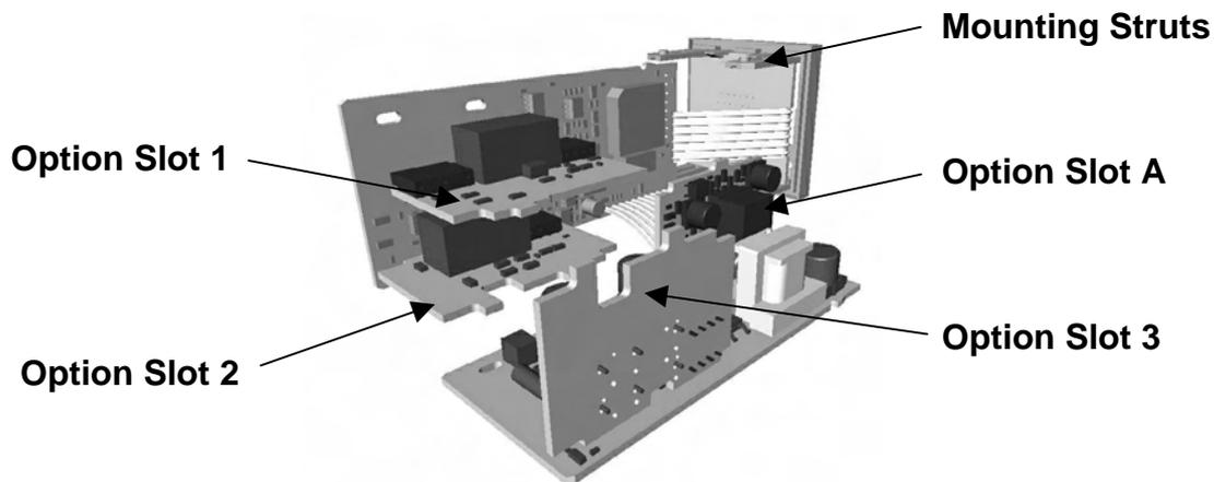
Figure 5. Location of Option Modules -  $\frac{1}{16}$  DIN Instruments
