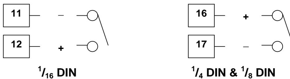
Figure 33. Option Slot A – Digital Input Module
