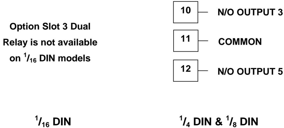
Figure 30. Option Slot 3 - Dual Relay Module
