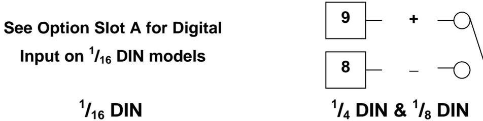
Figure 35. Option Slot B – Digital Input 2 Connections
