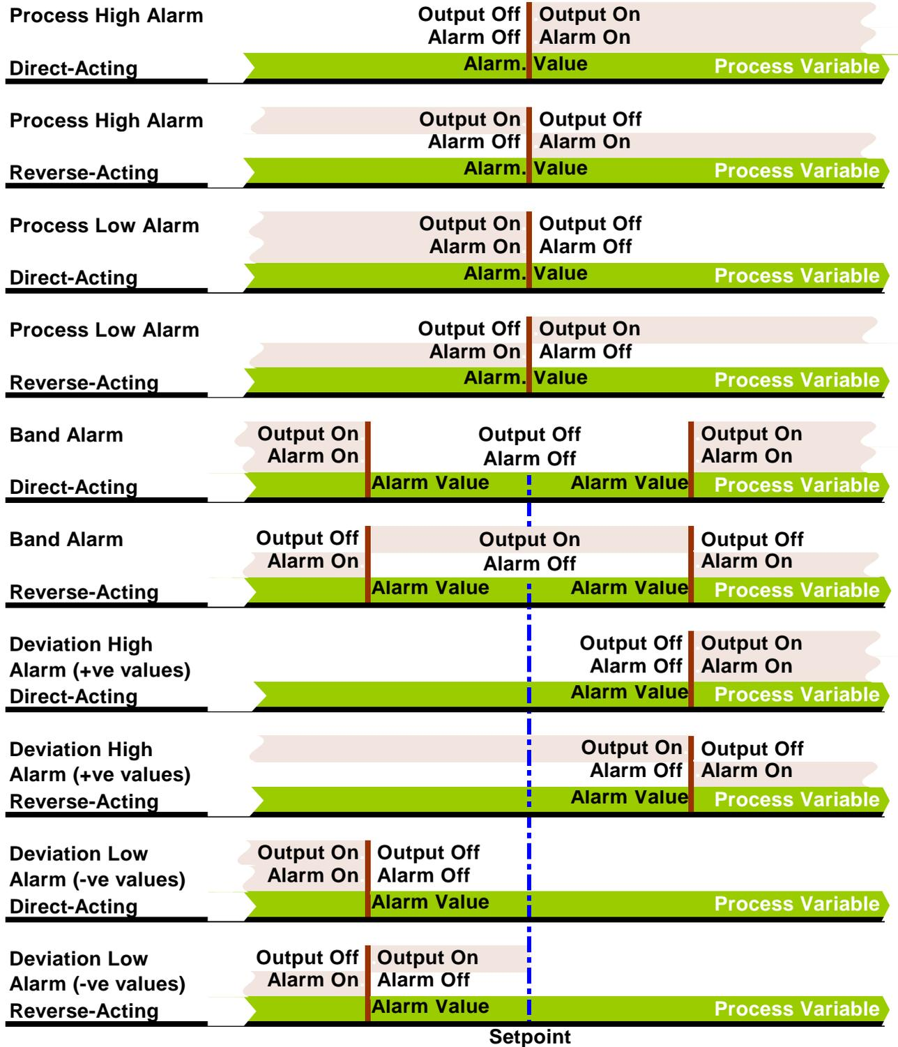
Figure 42. Alarm Operation
