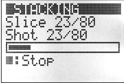
During a stack, the motorized stage will automatically move between slices, and shots will automatically be taken at the desired time interval. The current progress will be updated on the LCD after every shot taken. While the stacking controller is operating and photos are being taken, avoid touching the camera, subject, table, or apparatus to prevent movement and vibrations.
