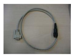
Connect the Programmer to the PC using the serial connection. Switch ON the programmer with the green button. The programmer now indicates that it is connected to the PC. The software will also indicate that it is connected.
