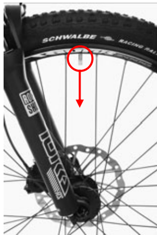
Valve pointing towards the middle of the wheel
