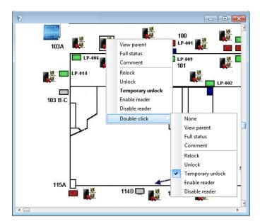
**NOTE:** Components in alarms are represented by their animated icons. Selecting an animated icon and viewing its parent components allows operators to learn more about the "alarm condition".
