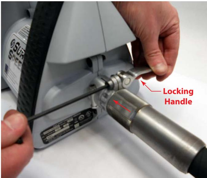
Figure 8: Locking lever adjustment
