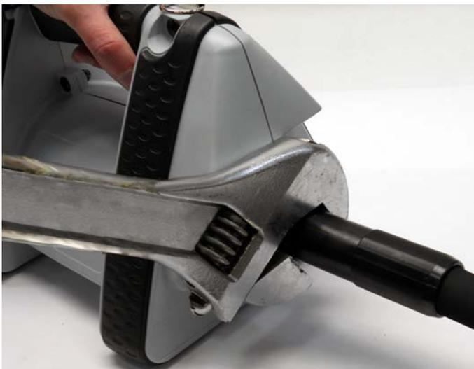
Figure 12: Hex motor connection
