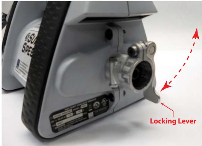
Figure 4: Quick disconnect fitting
