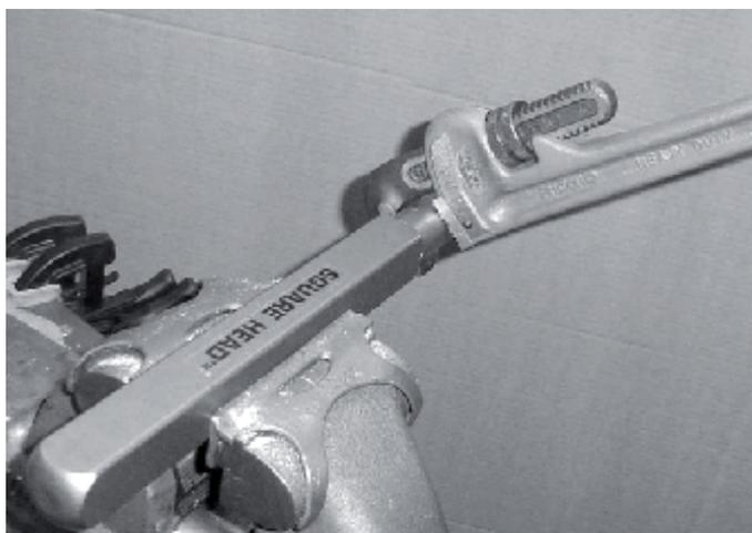
Figure 14: End cap removal
