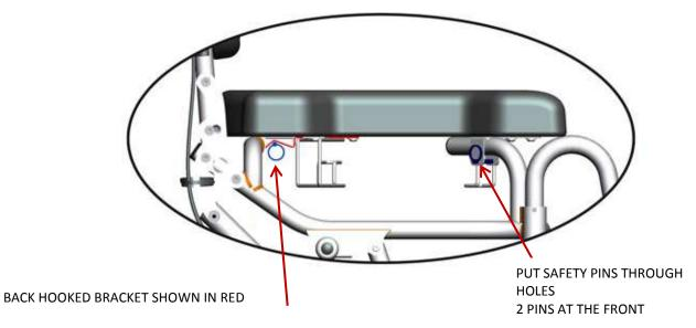
BRACKET HAS TO BE ENGAGED WITH THE SAFETY PIN PRESENTED IN BLUE
