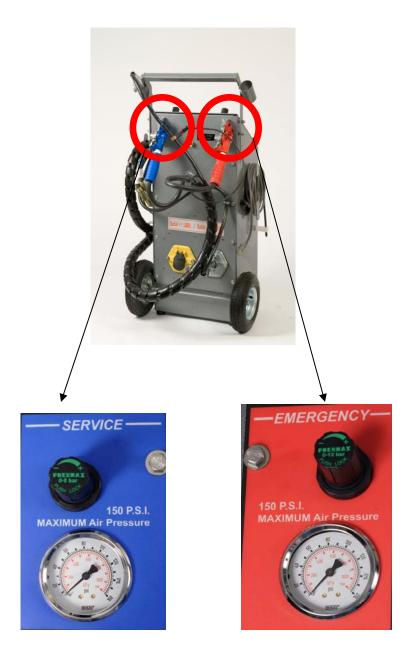
Two gladhands are installed on the back of the unit.
