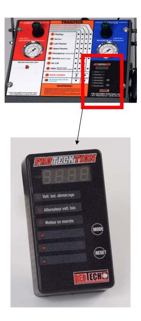
The circuit analyser on the TRAILteck unit has several functions. The "MODE" button activates each of the system's functions one at a time. This is very useful for detecting and repairing short circuits. This digital multimeter will become an indispensable tool in any mechanic's arsenal.
