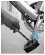
**Pedals** Pedals are marked "L" and "R" for left and right respectively. Screw in clockwise for the "R" pedal and counter-clockwise for "L". Tighten both with a wrench firmly but not excessively as the crank threads are made of aluminum alloy.
