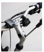
Handlebar / Stem / Headset Handlebar and stem comes pre-assembled. Loosen bolts on the stem and insert and turn the handle bar assembly until it is in right angles with the frame. Then tighten.
