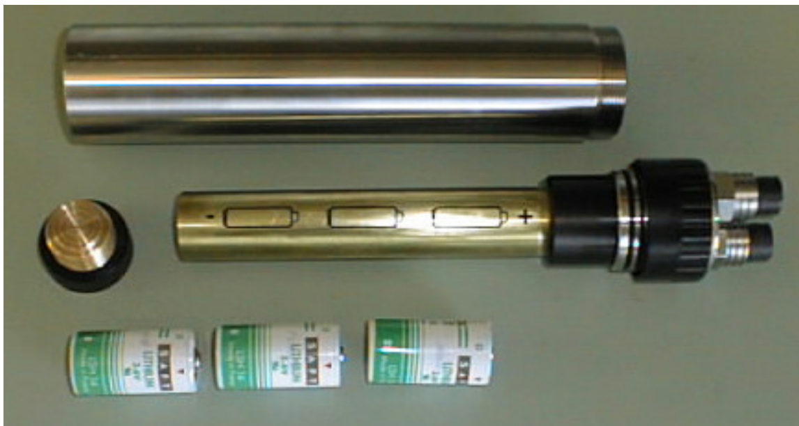
Figure 4.3.2.1 The Battery pack
