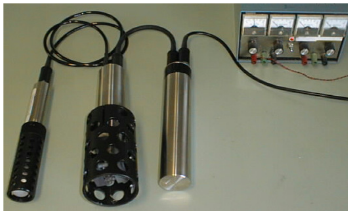
Figure 4.3.2 Micro instrument with battery pack and external sensor connected to external power
