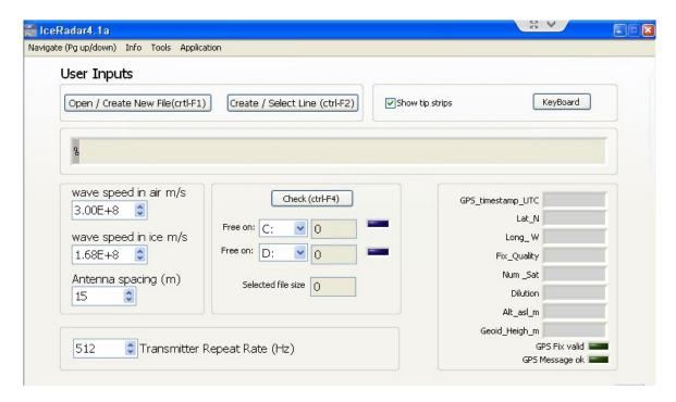
The User Inputs window allows the user to input the **Wave Parameters**, notably the **wave velocity in air**, the **wave velocity in ice**, and the **antenna spacing**.
