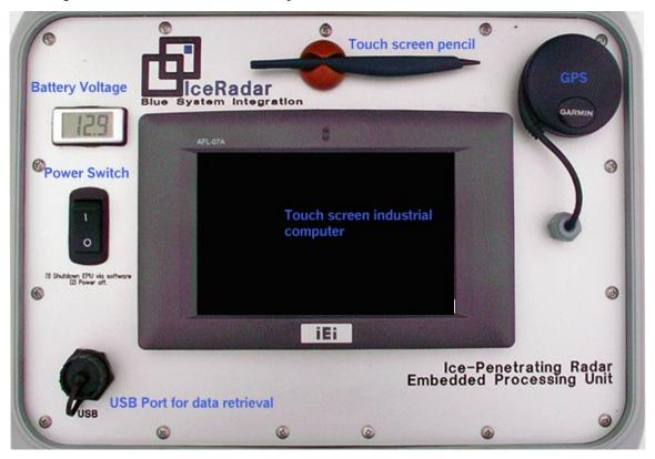
**Important:** To power down the system, **never** turn off the power switch before **first** shutting down the computer via software.
