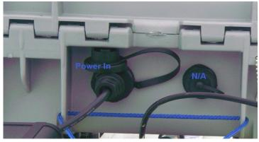
As soon as a power source is connected to the EPU, the voltage indicator should display a voltage reading. At this point turning the switch ON will boot the computer.
