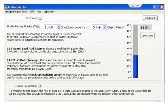
**Shutdown Level** specifies at which battery level the software will initiates and orderly shutdown. The battery level is checked at interval sets by the **Check Period**. **Enable Data Backup** insures there is always a second data file in the system updated at most 10 minute prior to the current data file. Check hard disk file available file space, as the backup procedure requires extra disk space.
