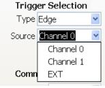
use the **EXT** input that is the lowest TNC input in the back of the EPU.
