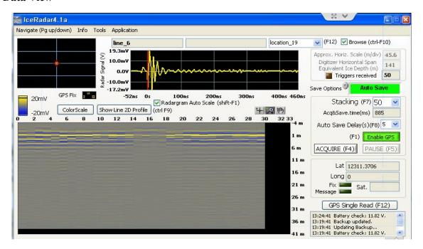
Select the **Save Options**, first to **No Data Save** to check the signal and fine tune the triggering. You can hit Acquire a few times to start building a 2D representation of the data. If **Single Point Save** is used, a **Create** / **Select Location pop-up** will appear to describe the given **Location**. Similarly to the Create / Select Line popup, a Location has a system name, given name, and description.
