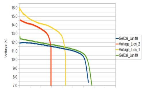
As a result it is very important to set up IceRadar Shutdown Level for the EPU well above the battery cut-off.
