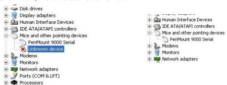
On next reboot, the system should not recognize the GPS as a ball mouse, and the unknown device should be gone. This issue is also detailed in the Garmin GPS documentation
