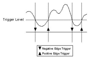
**Trigger Selection.Source** In IceRadar the Trigger typically uses the radar signal itself (air wave triggering), in this case use **channel 0** since the signal must be coming in on channel 0. Alternatively, some systems use a separate digital trigger with a fibre-optic setup installed between the transmitter and the receiver which would
