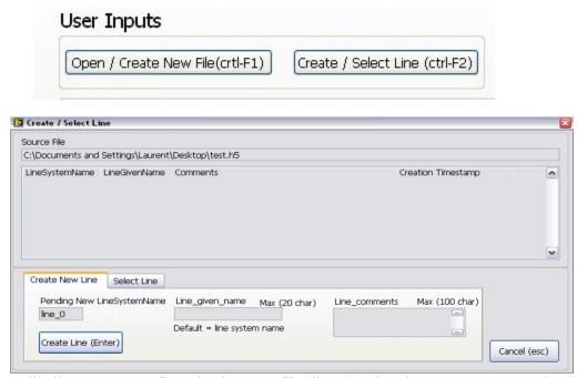
The above pop up will allow to create a first Line in a new file (line\_0). Lines have a system name that cannot be changed, a given name that is user-defined, and a comments attribute. Hit Create Line to create a new line. The new active line can be seen at the top of the Data View window above the radargram graph object.
