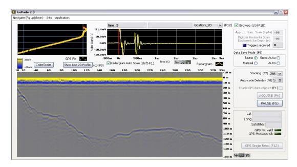
In other cases it may be more difficult to spot deeper bed reflections, in particular when one looks at a single radargram before the 2D data starts building up a profile.
