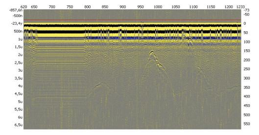
In some case, very little in terms of bed or internal reflections can be spotted, and only further filtering and data analysis will be able to provide a clear rendering of the data.
