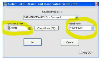
The Check Port button opens the Device Manager and is used for the Legacy NMEA\_GPS option when such devices were connected to a USB port on the computer. These required to find which serial port was associated with the GPS. This is not required when using the on-board Garmin GPS.
