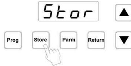
Continue through the parameter list by pressing the **PARM** button and making changes to the settings where needed. Follow the same procedure shown in steps 4 to 6 above.
