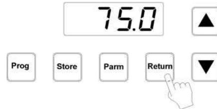
**NOTE:** If the AEC-2 is left displaying a parameter it will revert back to normal operation in 1 minute automatically. If **STORE** was not pressed the displayed parameter will change back to its previous value.
